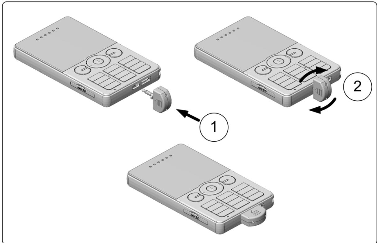
Insert Headset plug at 90 degree angle as figure above. Rotate the headset plug 90 degree to the right to lock the headset in the phone. To remove the headset, turn the headset plug left 90 degree then pull the headset out.
