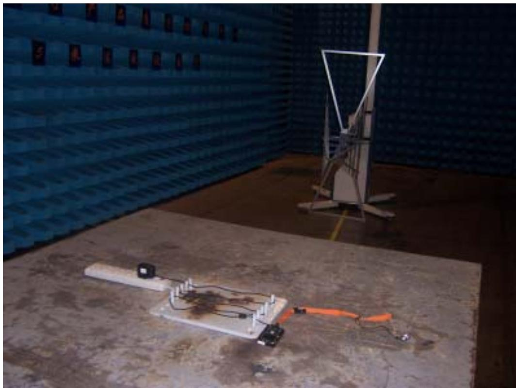
**4. Radiated Emission Test, USB Mode**
