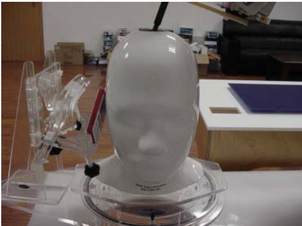
Fig.6 EUT Right Head Tilt15 Position
