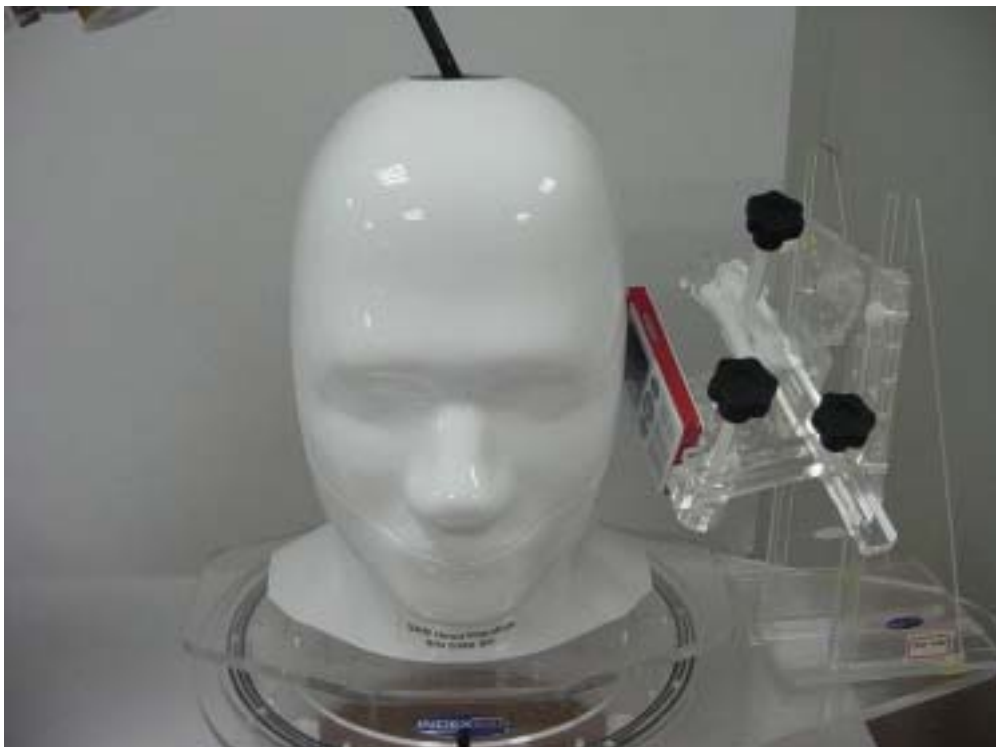
Fig.4 EUT Left Head Tilt15 Position
