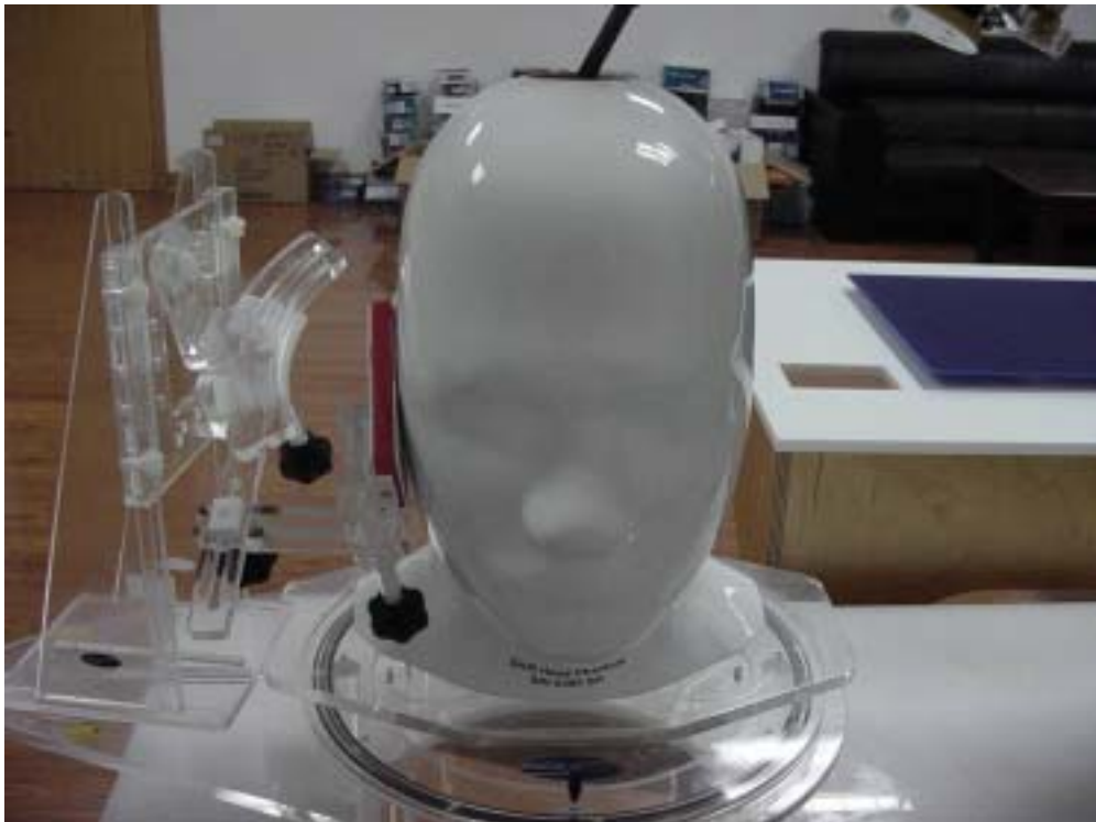
Fig.5 EUT Right Head Touch Cheek Position
