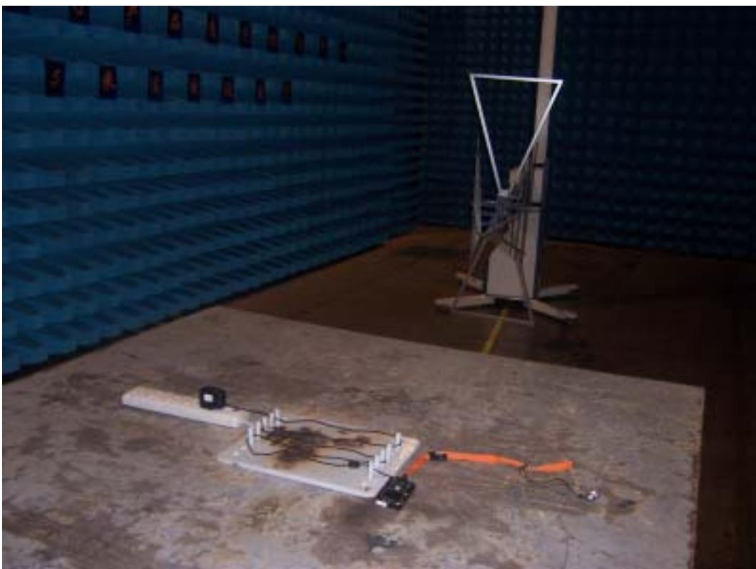
**4. Radiated Emission Test, USB Mode**
