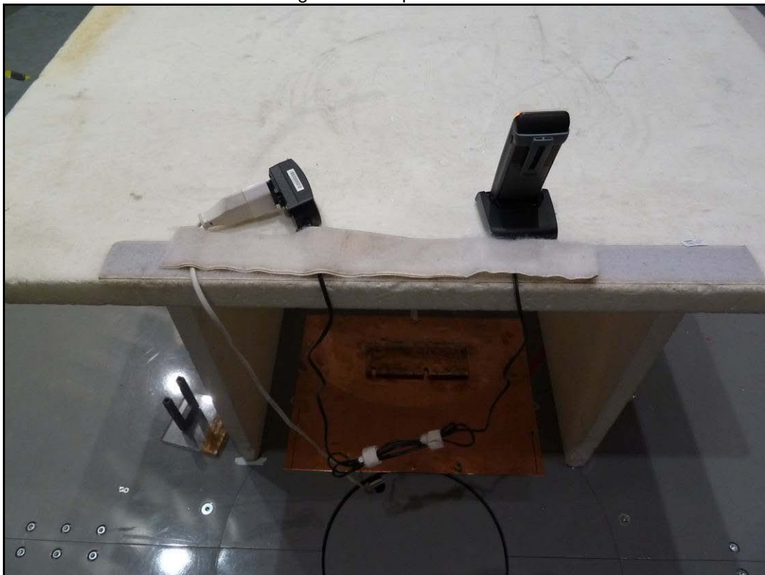
Photo 4: wiring of the setup of radiated emission
