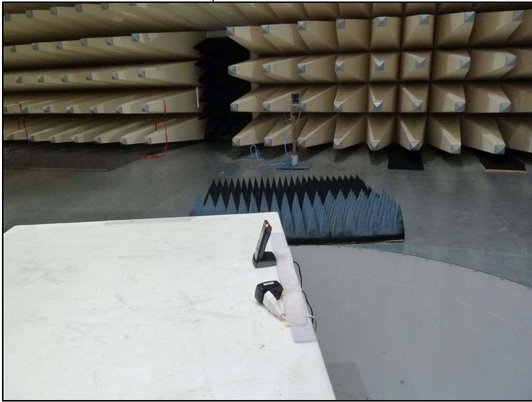
Photo 4: wiring of the setup of radiated emission
