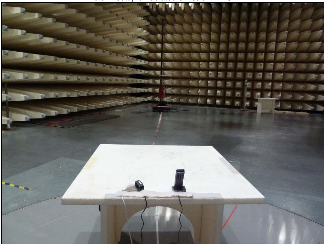
Photo 2: setup of radiated emission < 1 GHz
