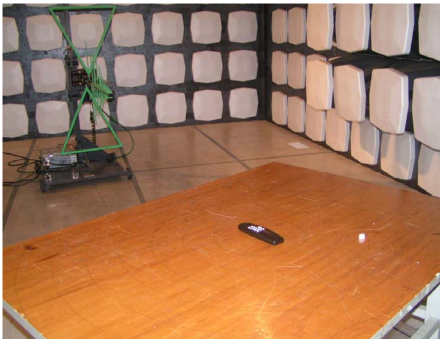
Field Strength Emissions Test Set-up (Below 1GHz)
