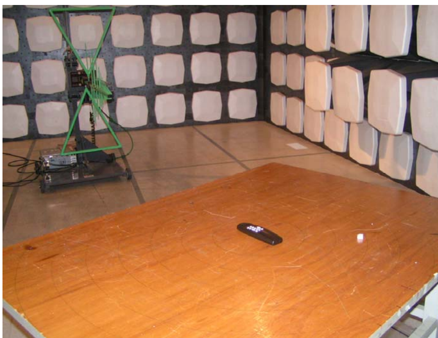
Field Strength Emissions Test Set-up – Rear View (Below 1GHz)
