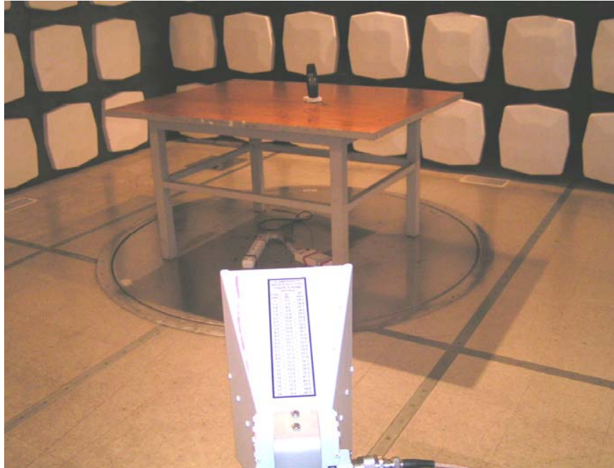
Field Strength Emissions Test Set-up – Front View (Above 1GHz)
