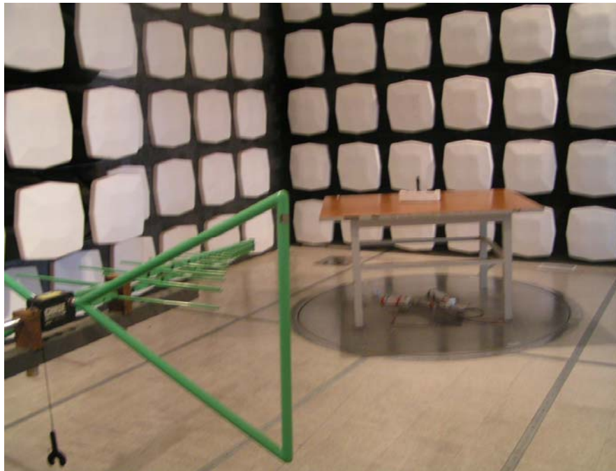
Field Strength Emissions Test Set-up – Front View (Below 1GHz)
