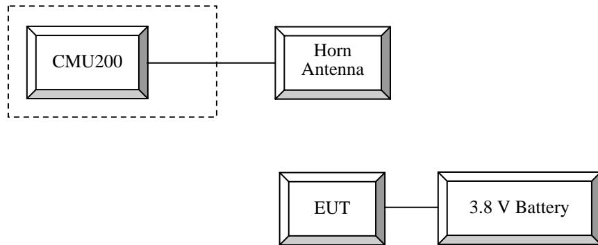
**Block Diagram of Test Setup**
