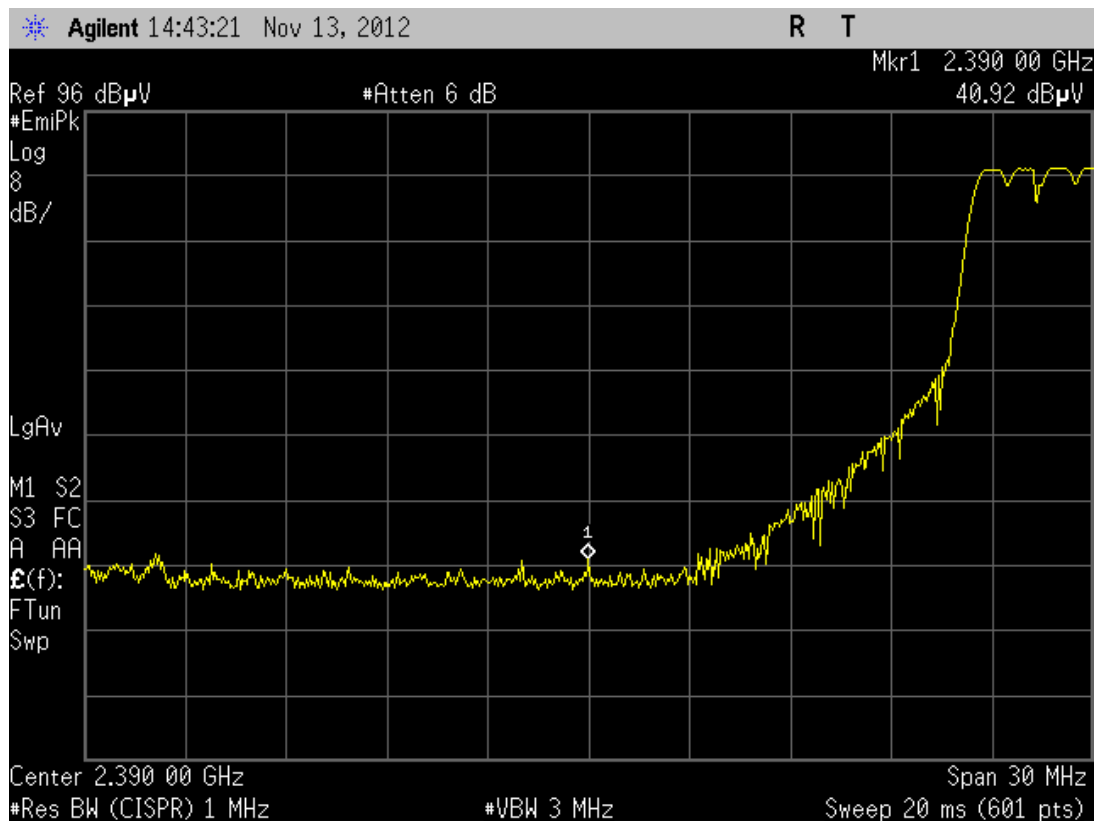
Figure 4. Hopping on, Band-edge compliance, low end
