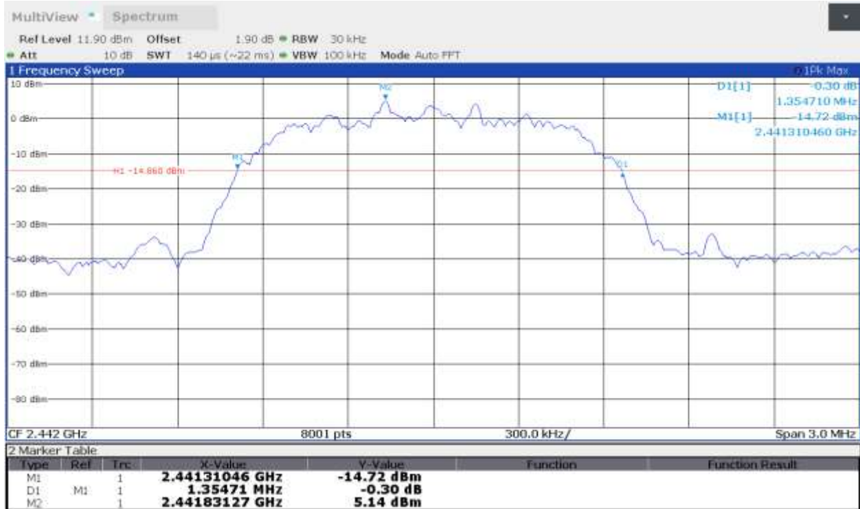
Plot 1.5 – 20dB Bandwidth and 99% Bandwidth, \pi/4 -DQPSK, 2442 MHz
