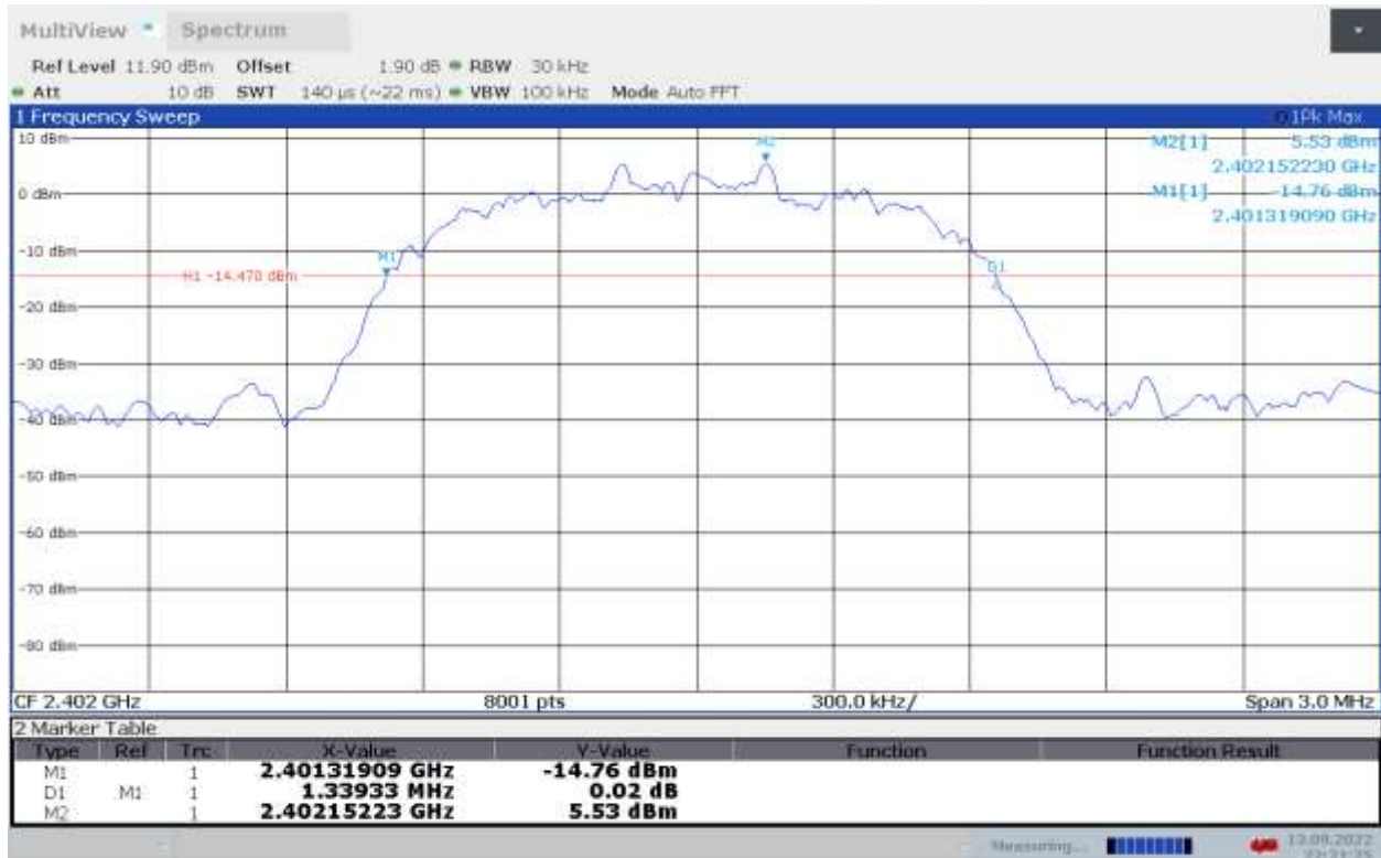
Plot 1.7 – 20dB Bandwidth and 99% Bandwidth, 8-DPSK, 2402 MHz
