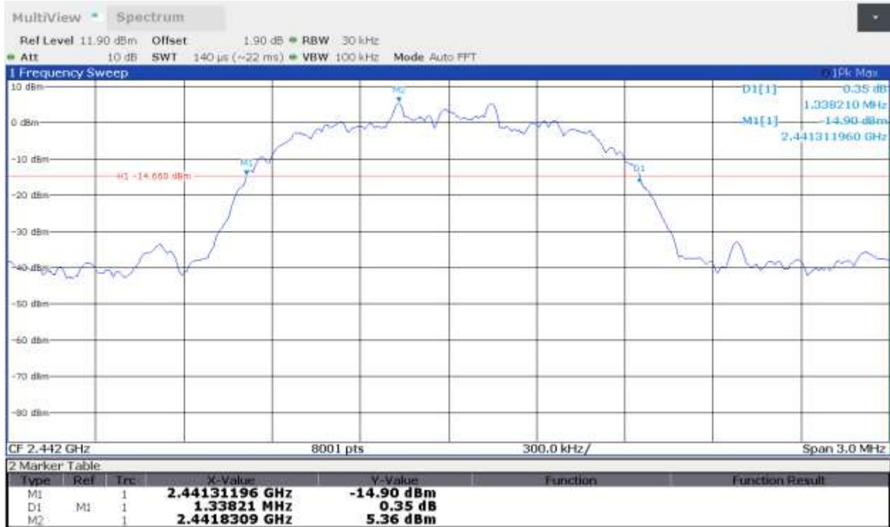
Plot 1.8 – 20dB Bandwidth and 99% Bandwidth, 8-DPSK, 2442 MHz
