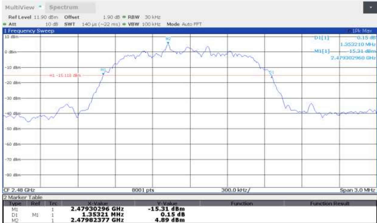
Plot 1.6 – 20dB Bandwidth and 99% Bandwidth, \pi/4 -DQPSK, 2480 MHz
