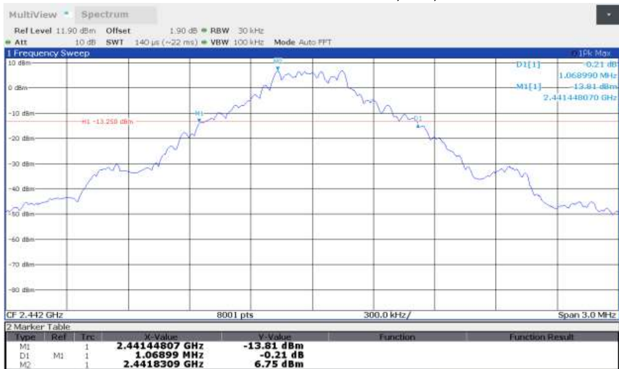
Plot 1.2 – 20dB Bandwidth and 99% Bandwidth, GFSK, 2442 MHz
