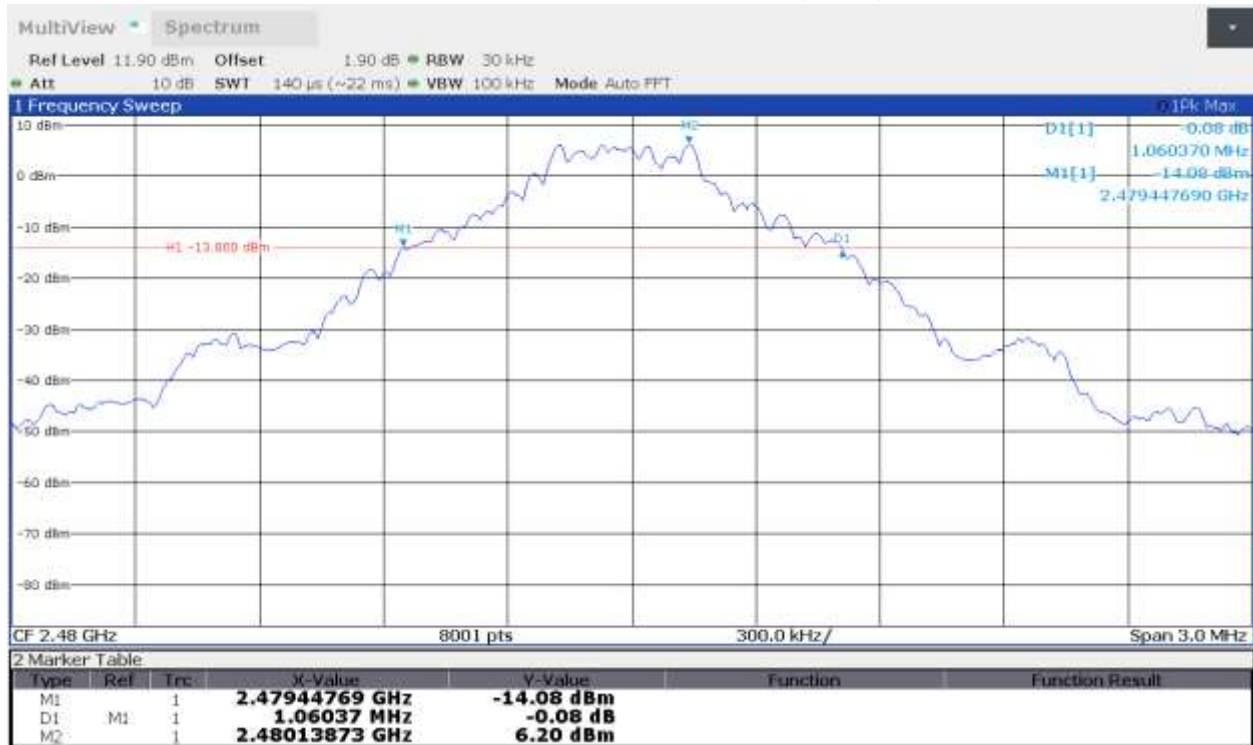
Plot 1.3 – 20dB Bandwidth and 99% Bandwidth, GFSK, 2480 MHz
