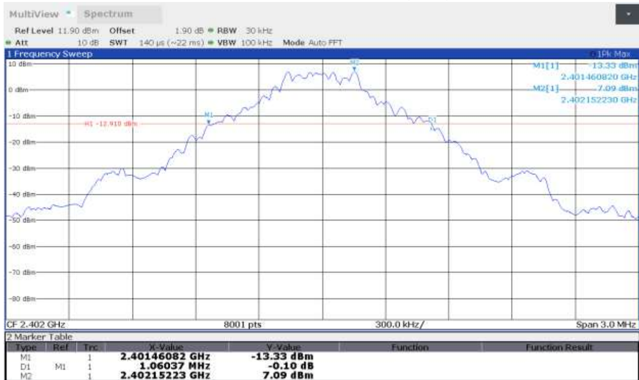
Plot 1.1– 20dB Bandwidth and 99% Bandwidth, GFSK, 2402 MHz
