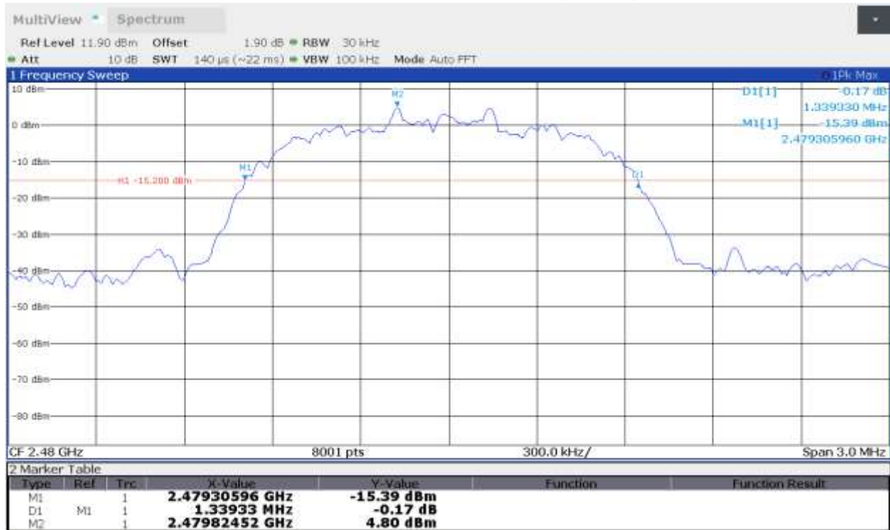
Plot 1.9 – 20dB Bandwidth and 99% Bandwidth, 8-DPSK, 2480 MHz
