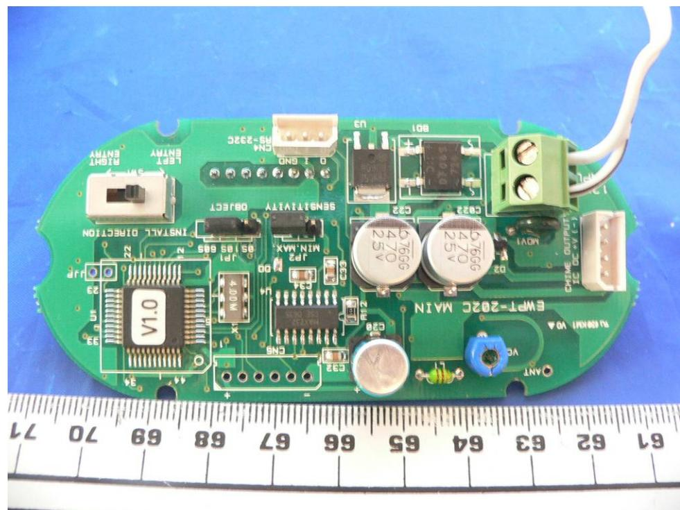
**EUT Main PCB Board Side Two View**
