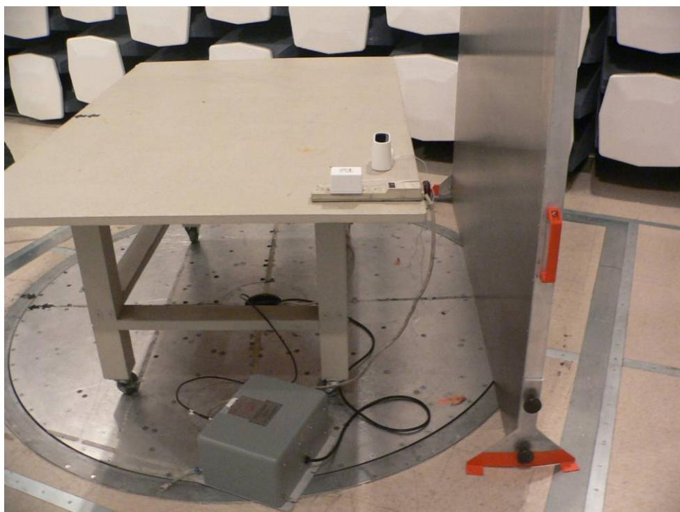
**Radiated Emissions - Front View**
