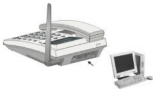
Figure 4-5 Connecting the FWT to a PC through a serial communication cable
