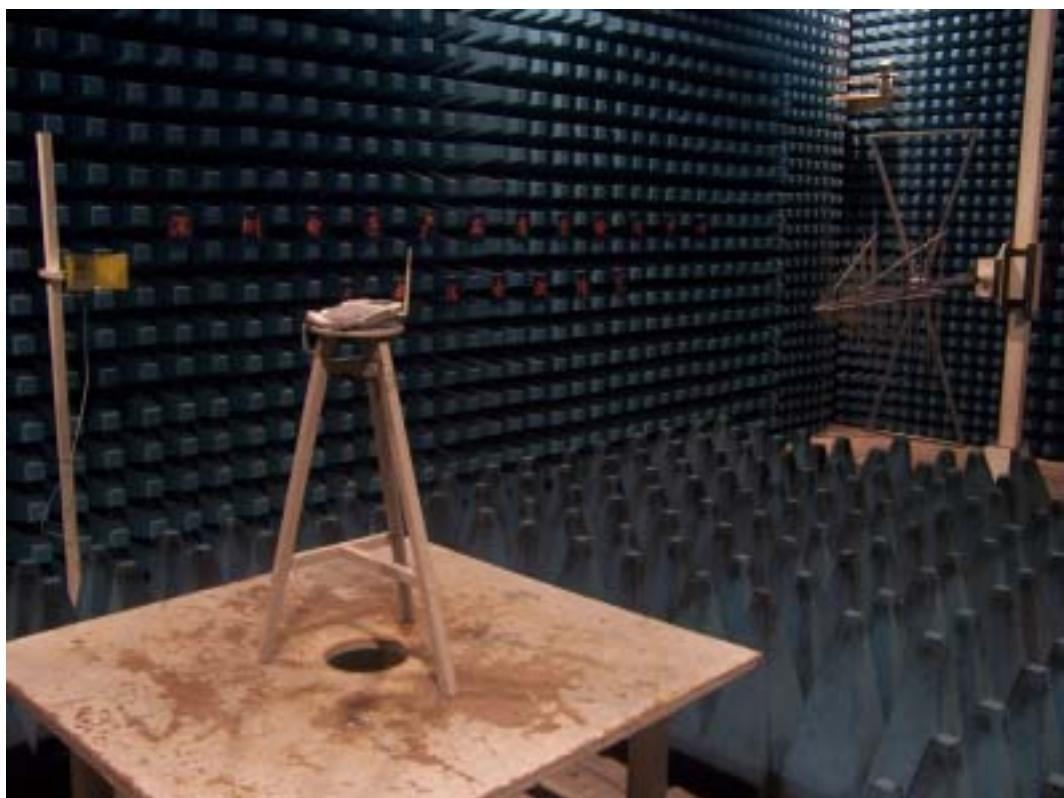
**7. Radiated RF Test (9kHz~30MHz)**
