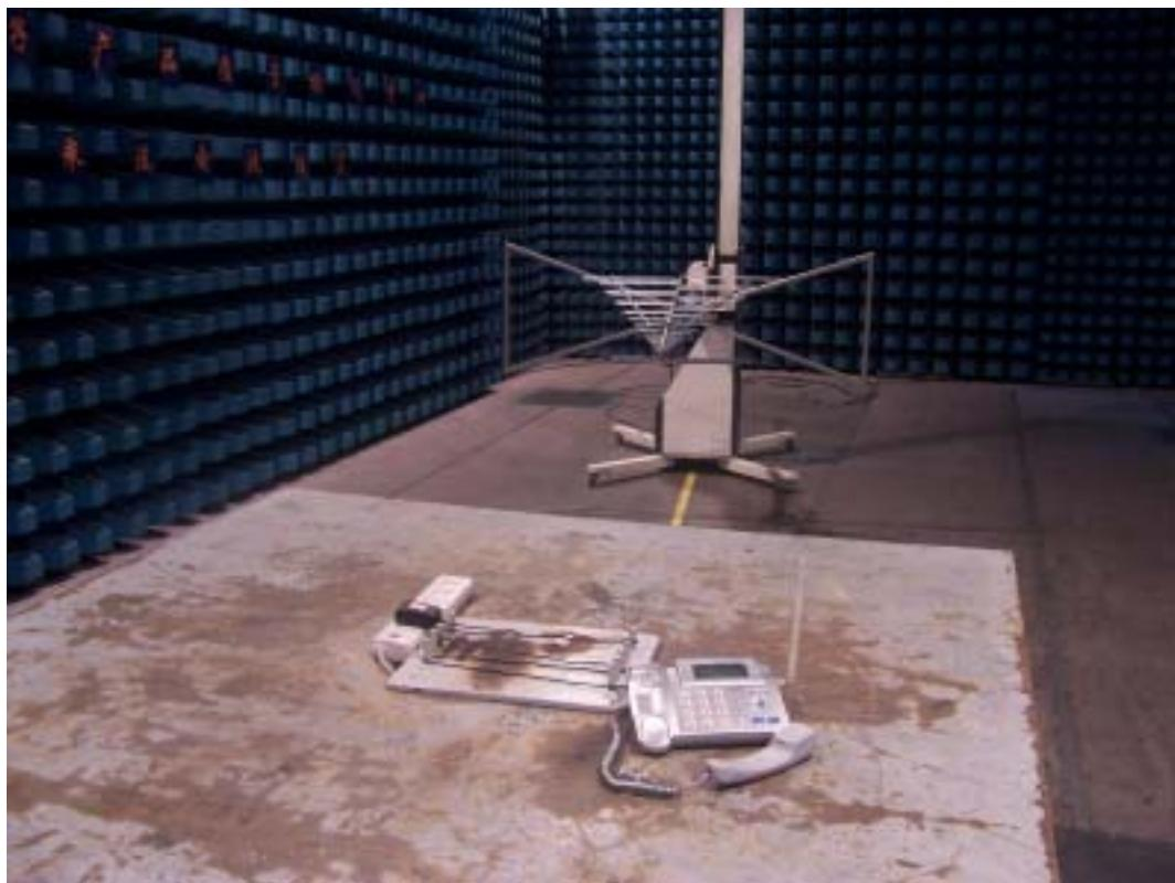
**4. Radiated Emission Test (Data Mode)**
