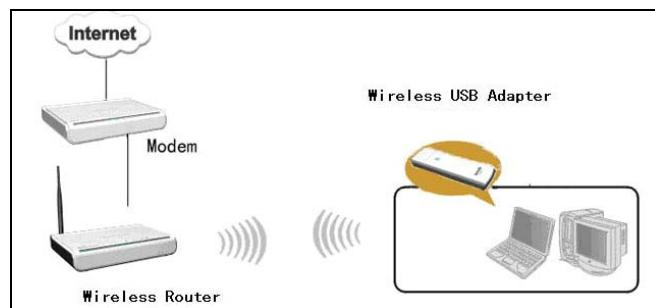
In this mode, MXP3802NU2C serves as a client to receive the wireless signals to access the Internet.
