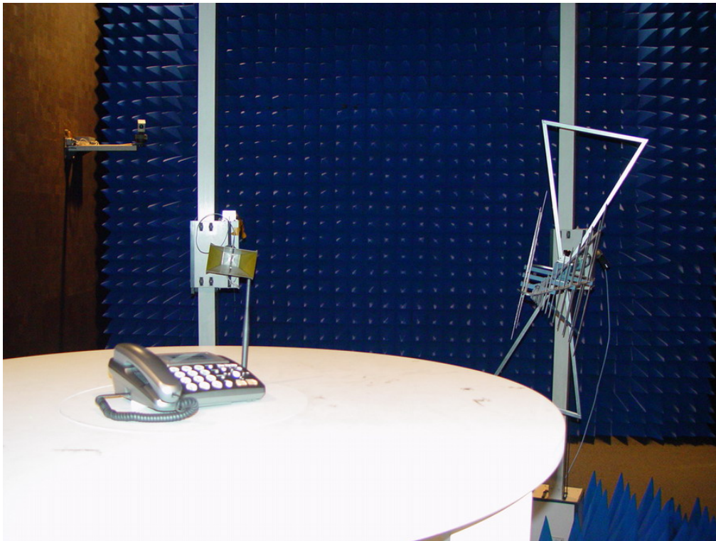
Pic 1 Radiated Spurious Emissions Test Setup
