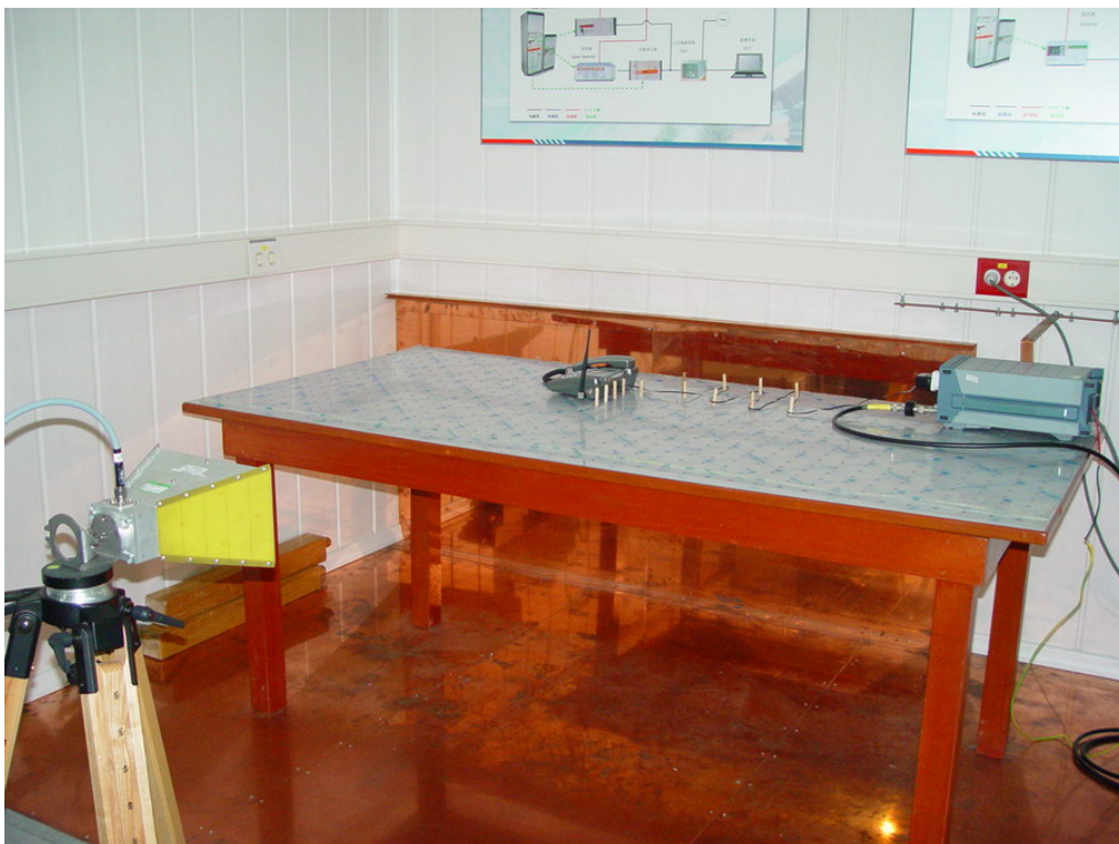
Pic 2 Conducted Emissions Test Setup
