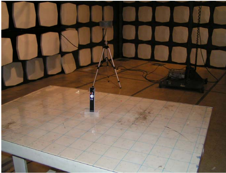
Radiated Emissions Test Set-up – Stand mode
