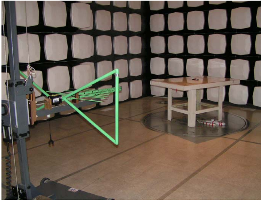
Radiated Emissions Test Set-up (Low frequency)
