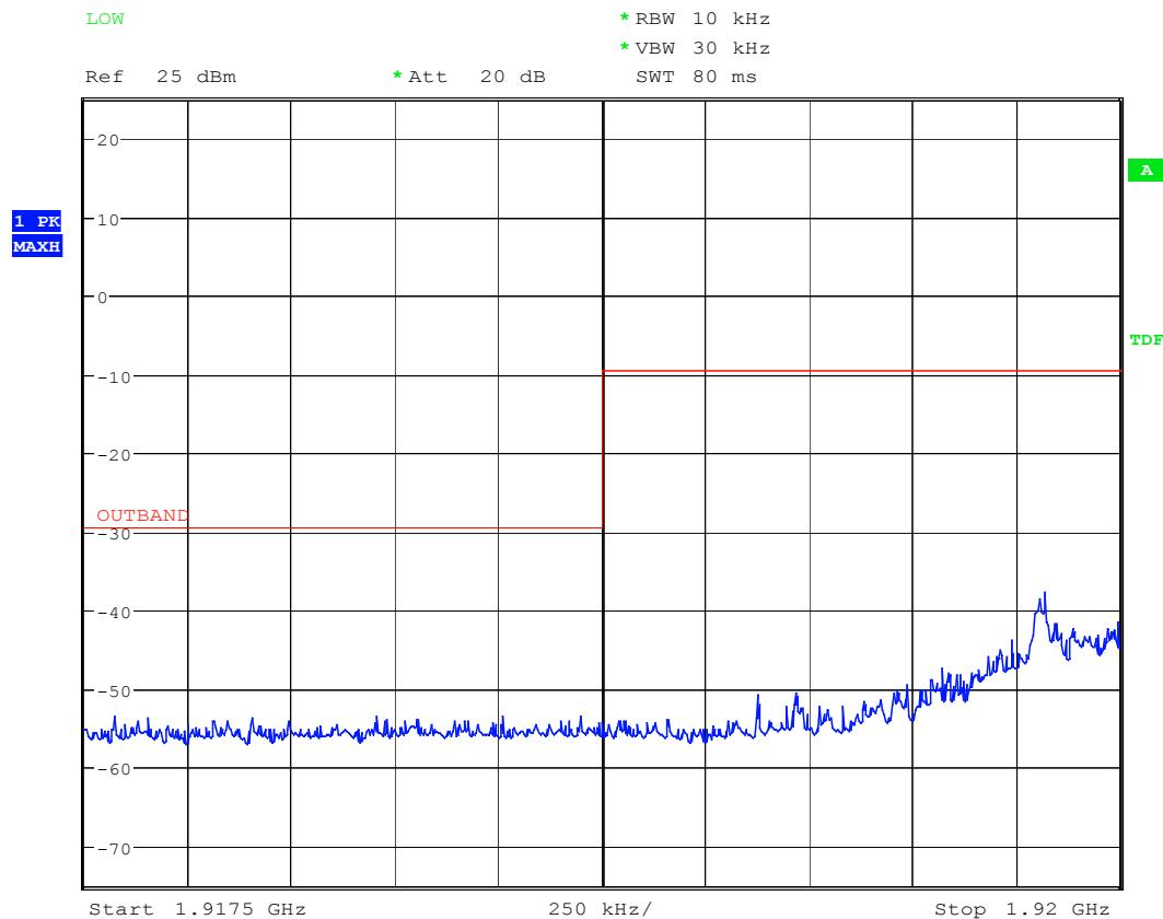
**Out-of-band Unwanted Emissions: CH F<sub>L</sub>**
