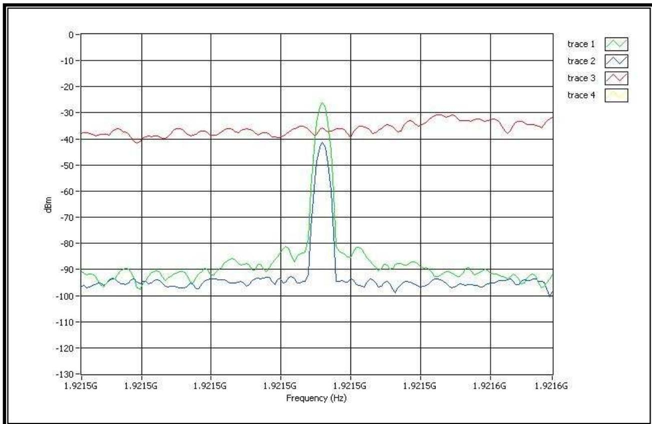
Note 1: Trace1 (green) is the interference on the carrier. The level is TU+UM+10dB.
