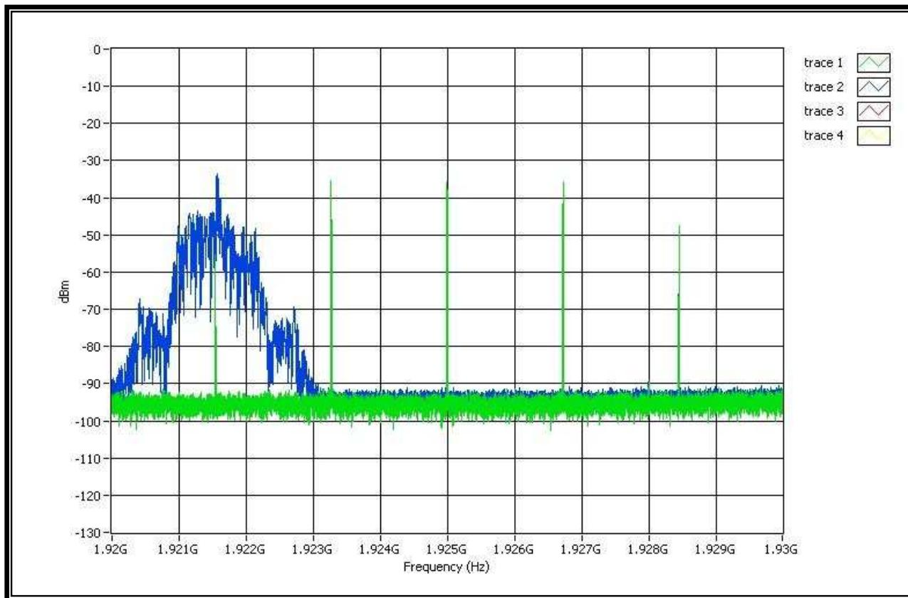
Note 1: The interference of level on f2 is TL+UM+7dB. The interference of level on f1 is TL+UM. The level of other 3 carriers is TU+UM.
