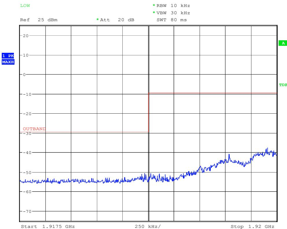
**Out-of-band Unwanted Emissions: CH F<sub>L</sub>**
