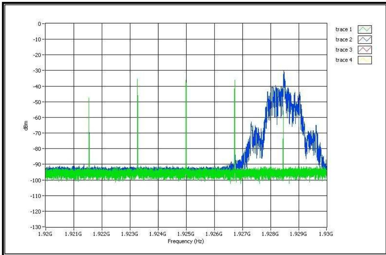
Note 1: The interference of level on f1 is TL+UM+7dB. The interference of level on f2 is TL+UM. The level of other 3 carriers is TU+UM.
