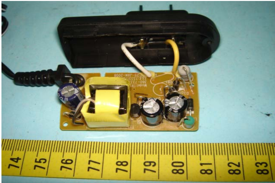
Component View of Adaptor's PCB
