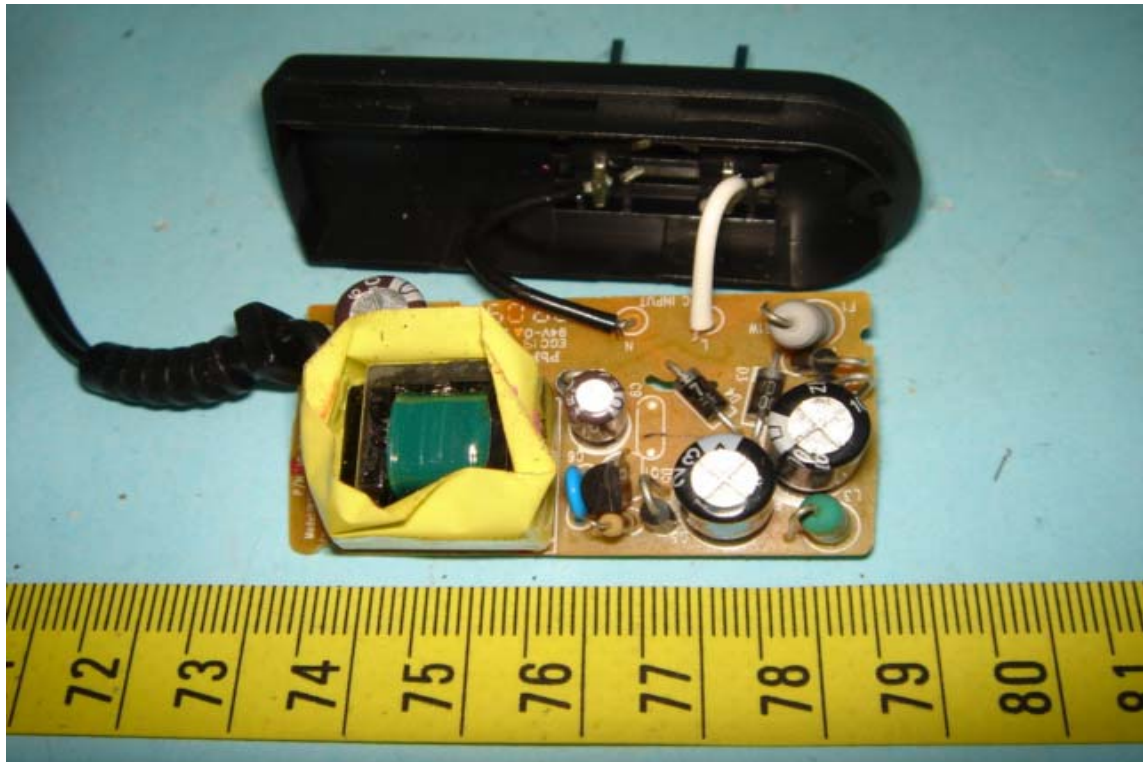
Component View of Adaptor's PCB
