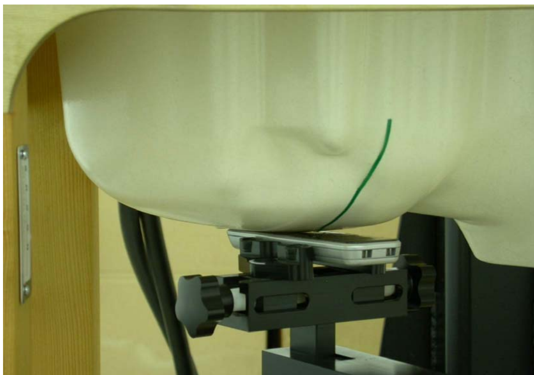
Measurement Position of Right-Cheek (RC) with Handset
