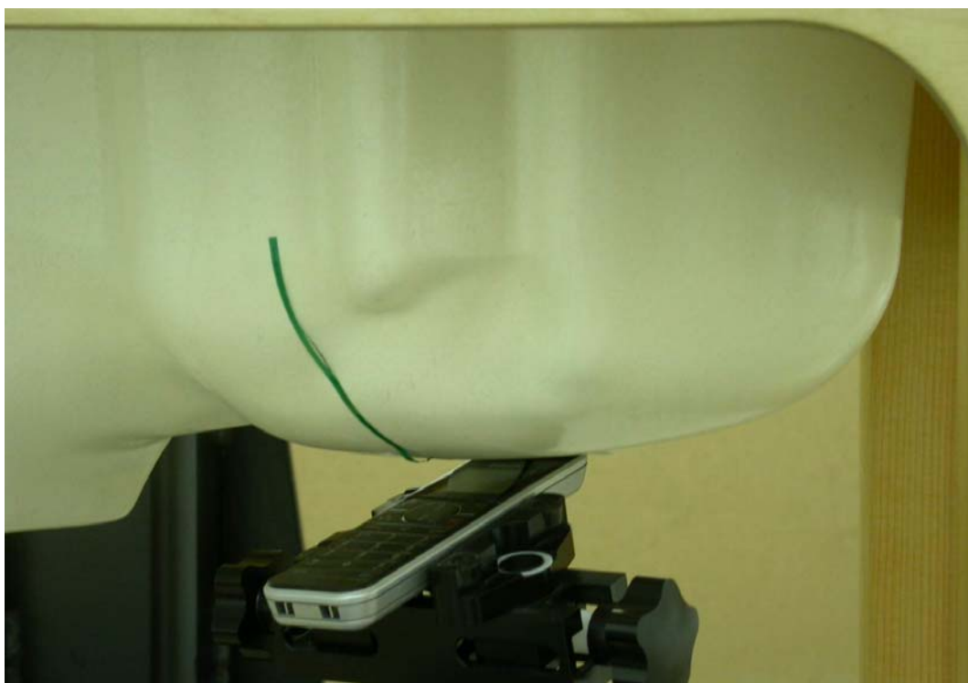
Measurement Position of Left-Tilt (LT) with Handset
