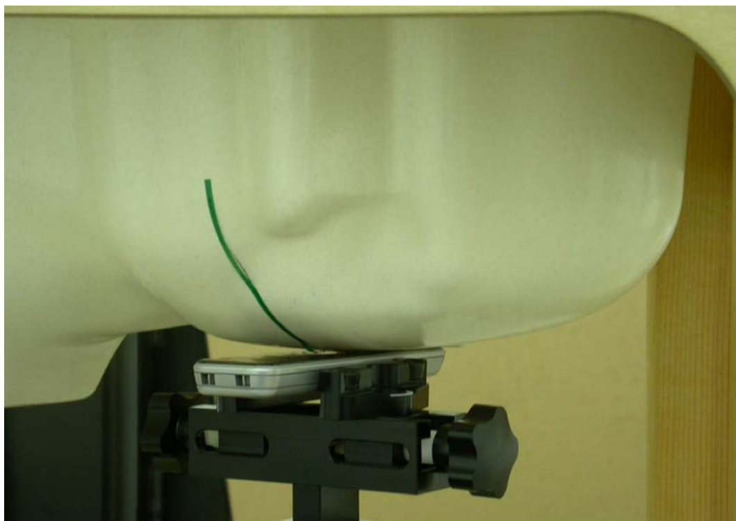
Measurement Position of Left-Cheek (LC) with Handset
