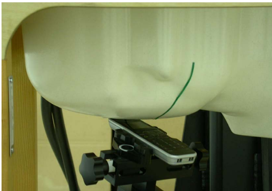
Measurement Position of Right-Tilt (RT) with Handset
