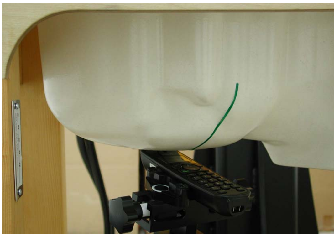
Measurement Position of Right-Tilt (RT) with Handset
