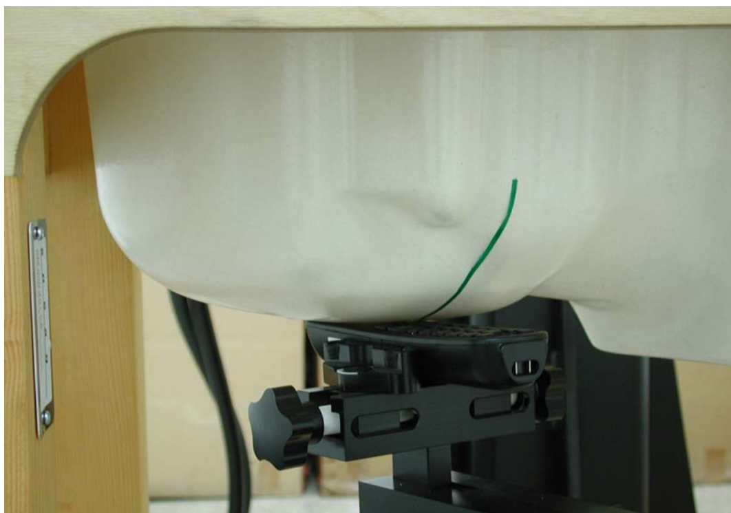
Measurement Position of Right-Cheek (RC) with Handset
