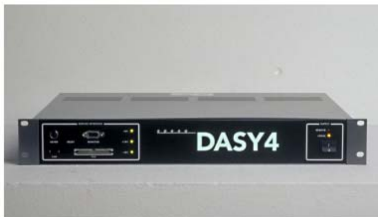
Fig. 7 DASY4 Measurement Server
