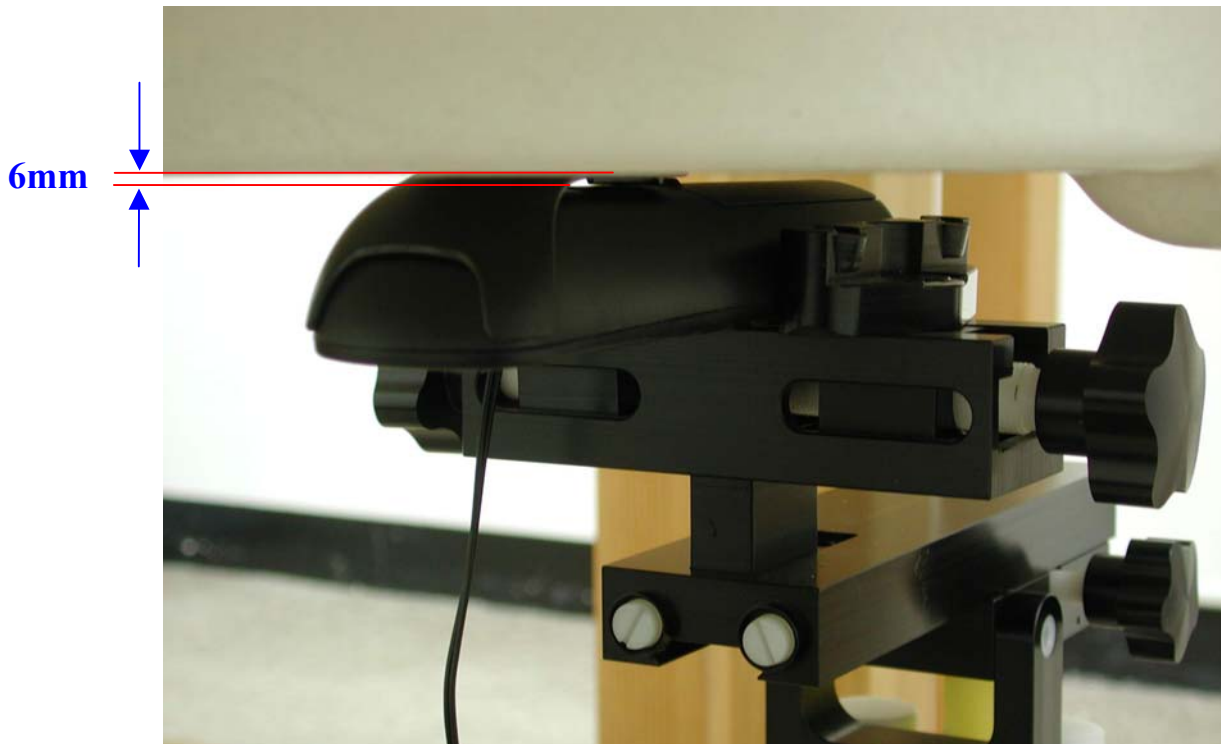
Measurement Position of Rear-UP with Handset
