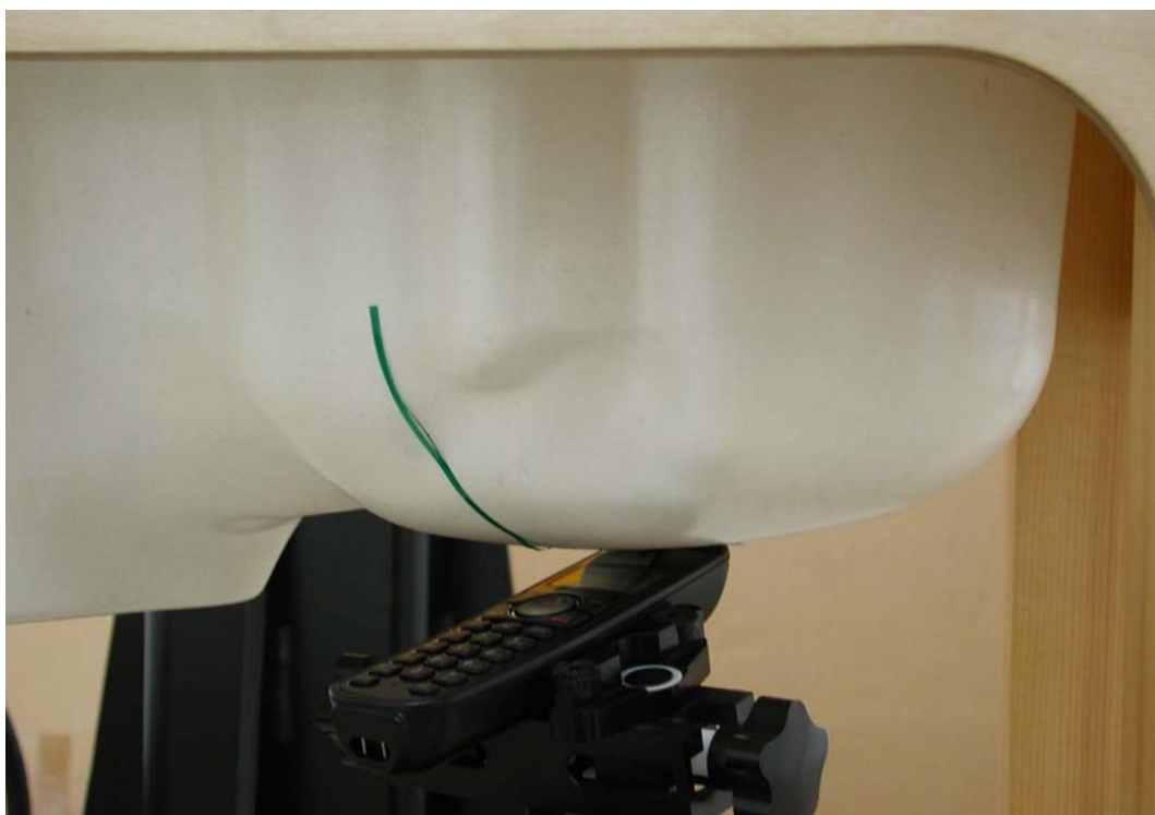
Measurement Position of Left-Tilt (LT) with Handset
