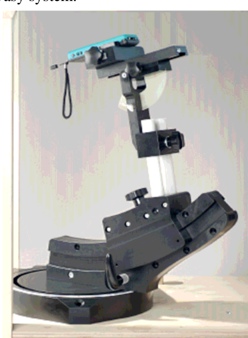
Fig. 10 Device holder supplied by SPEAG
