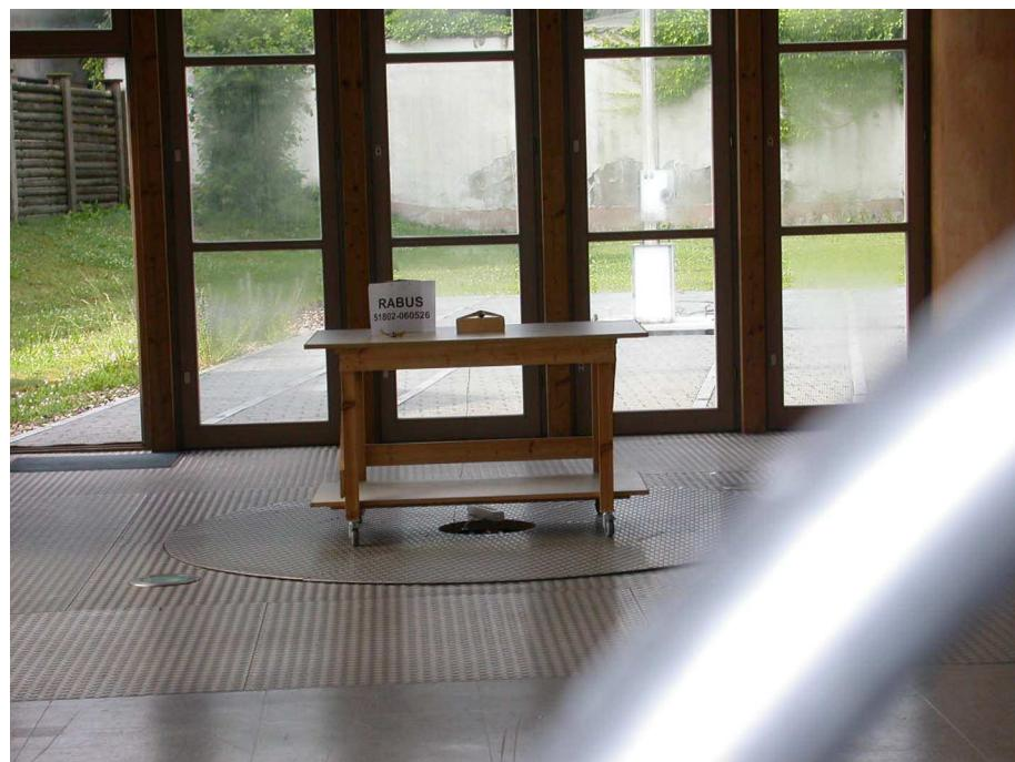
**Test setup for radiated emission measurement
