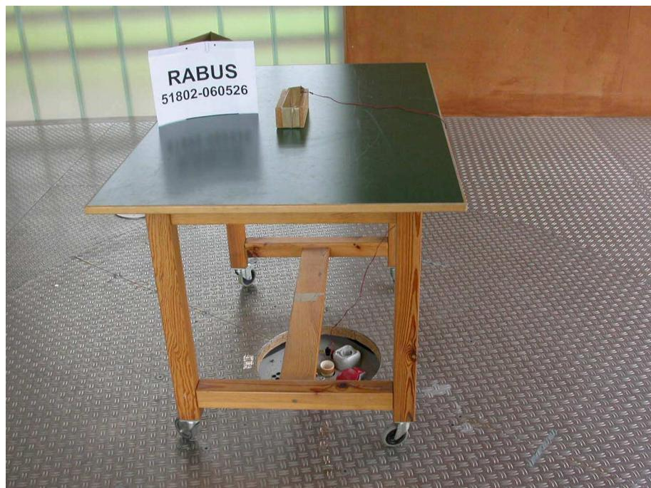
**Test setup for radiated emission measurement
