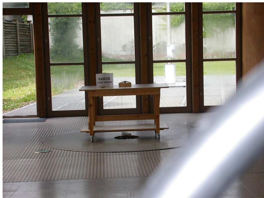
**Test setup for radiated emission measurement
