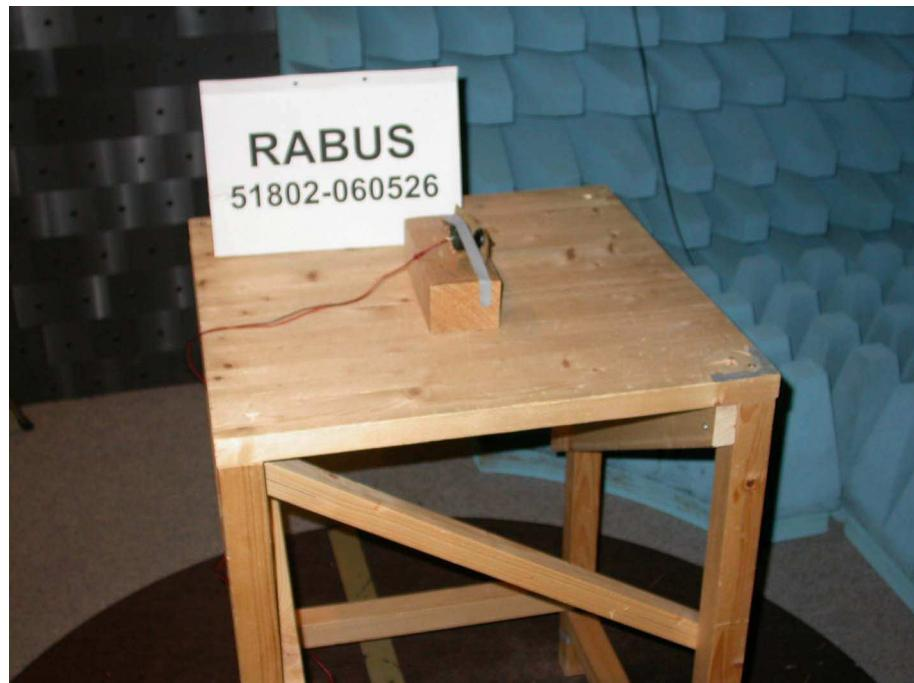
**Test setup for radiated emission measurement
