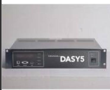
The DASY5 measurement server is based on a PC/104 CPU board with a 400MHz intel ULV celeron, 128MB chip-disk and 128 MB RAM. The necessary circuits for communication with either the DAE4(or DAE3) electronic box as well as the 16-bit AD-converter system for optical detection and digital I/O interface are contained on the DASY5 I/O-board, which is directly connected to the PC/104 bus of the CPU board.
