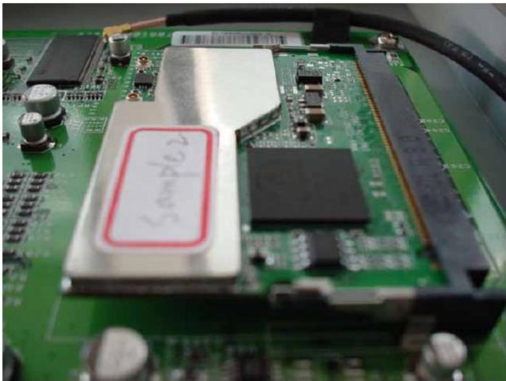
3. Connect the internal antenna
