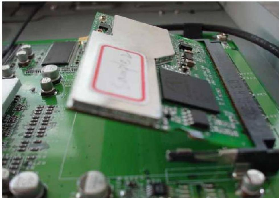
2. Press down the Mini-PCI and make sure the combination be firm.
