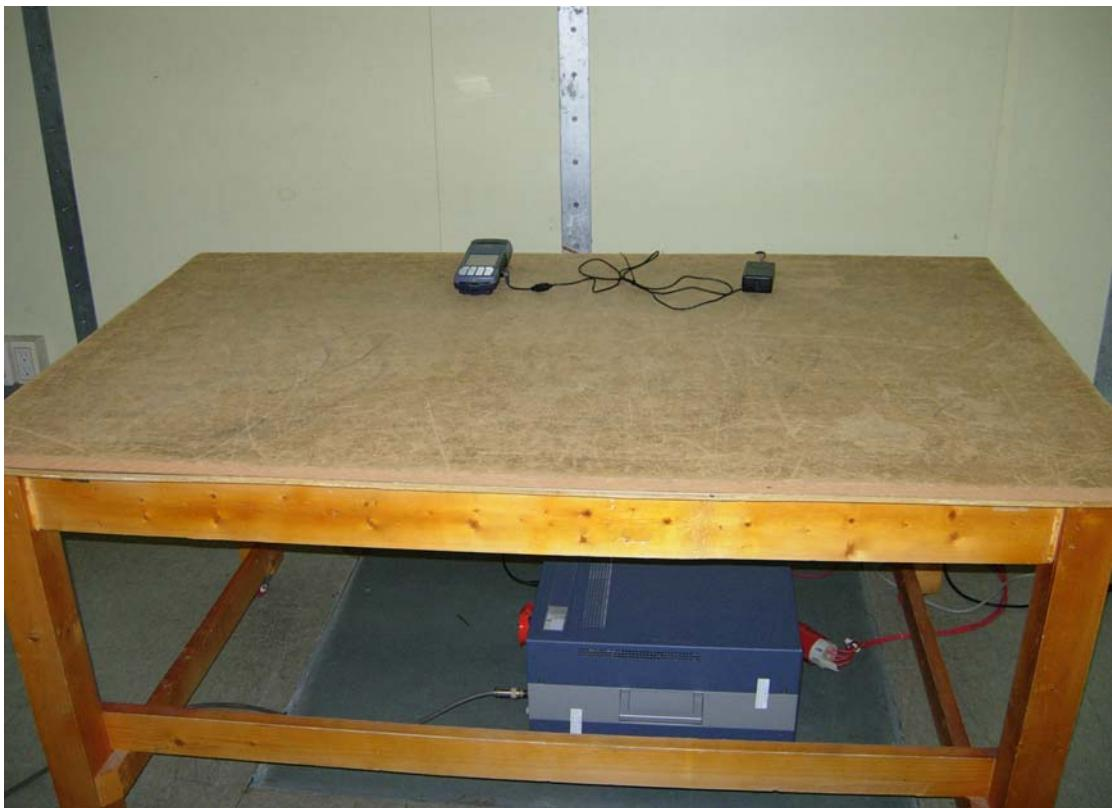
**<Conducted Emissions: Adaptor only – Rear View>**
