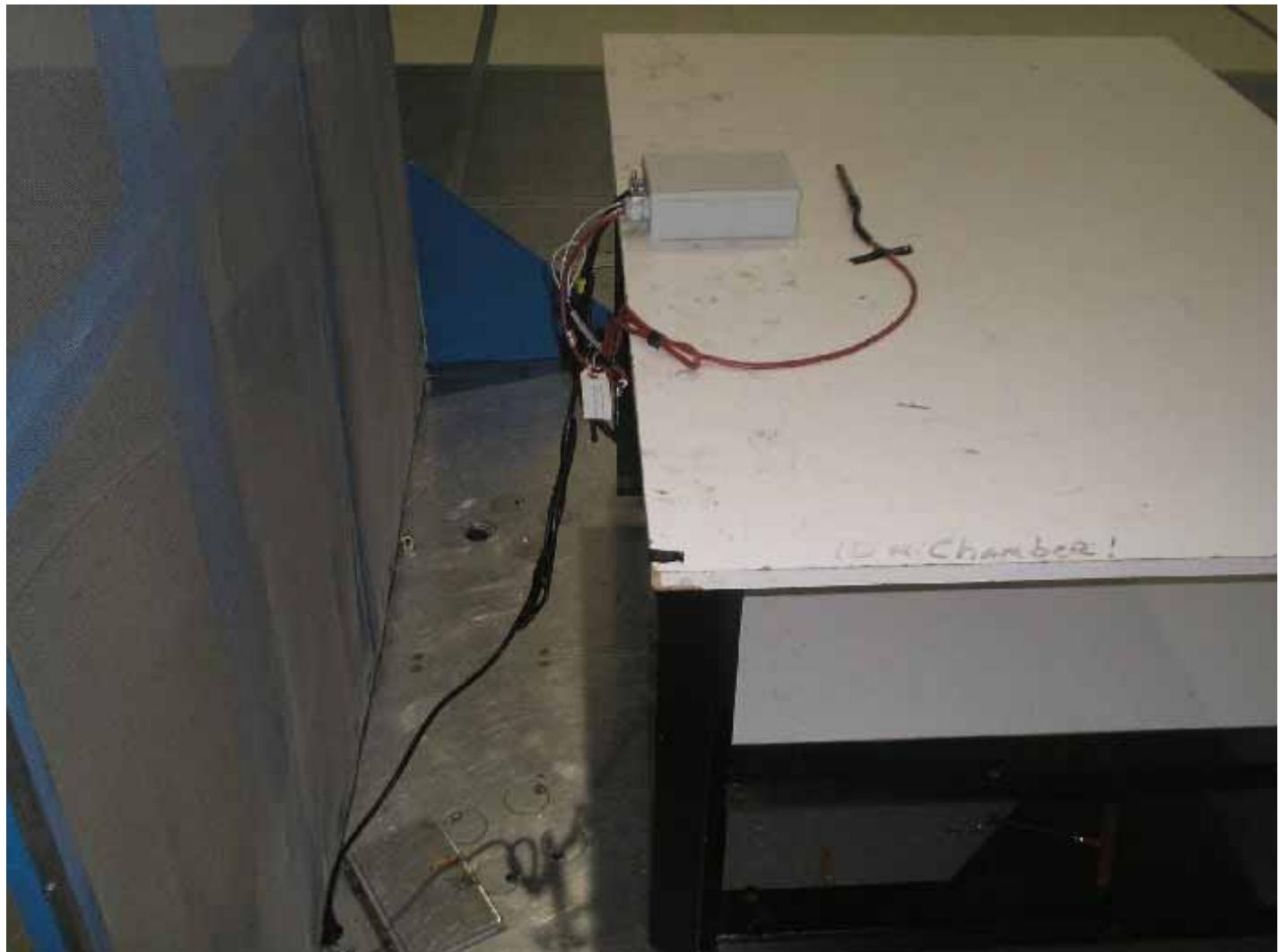
Conducted Emissions Rear Test Setup
