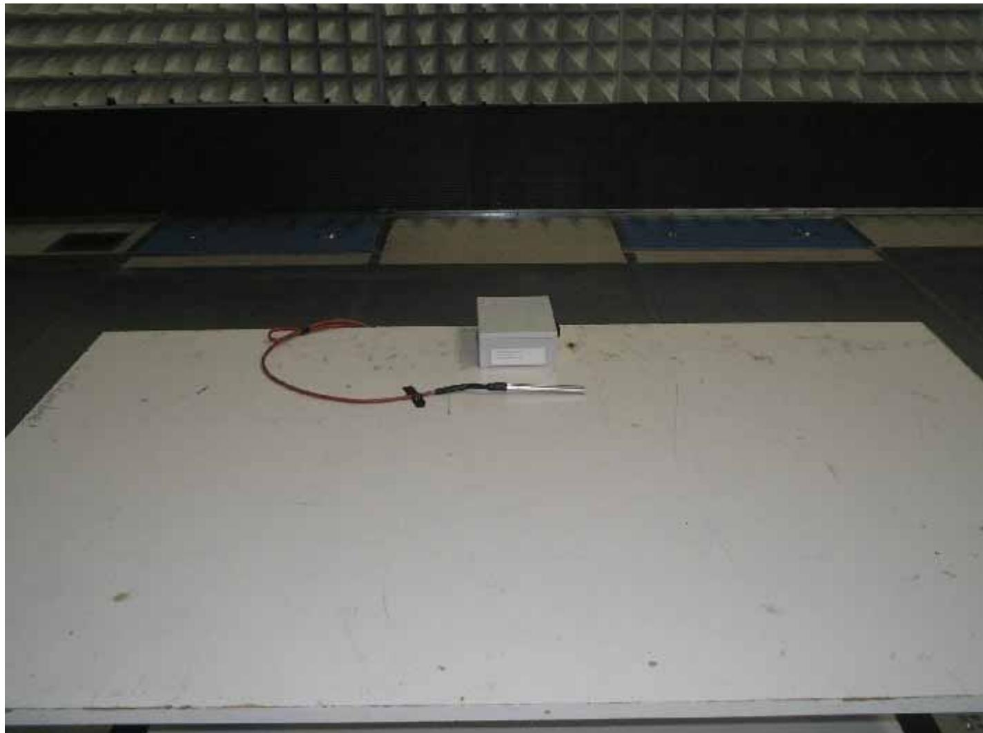
Radiated Emissions Front Test Setup
