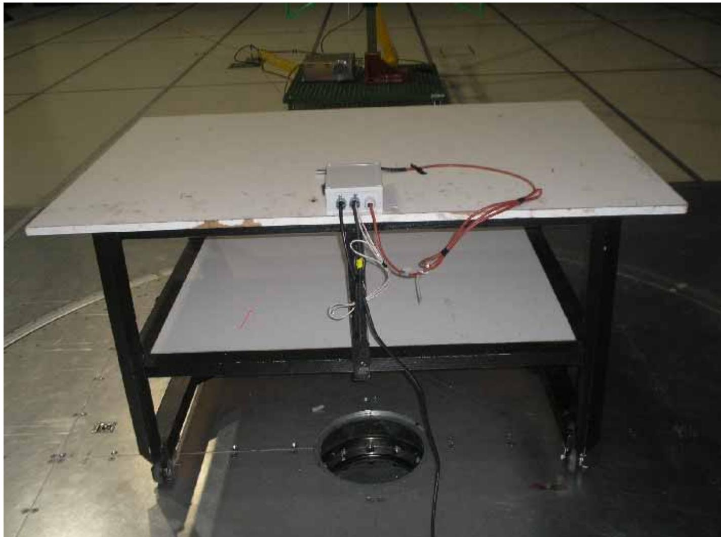
Radiated Emissions Rear Test Setup
