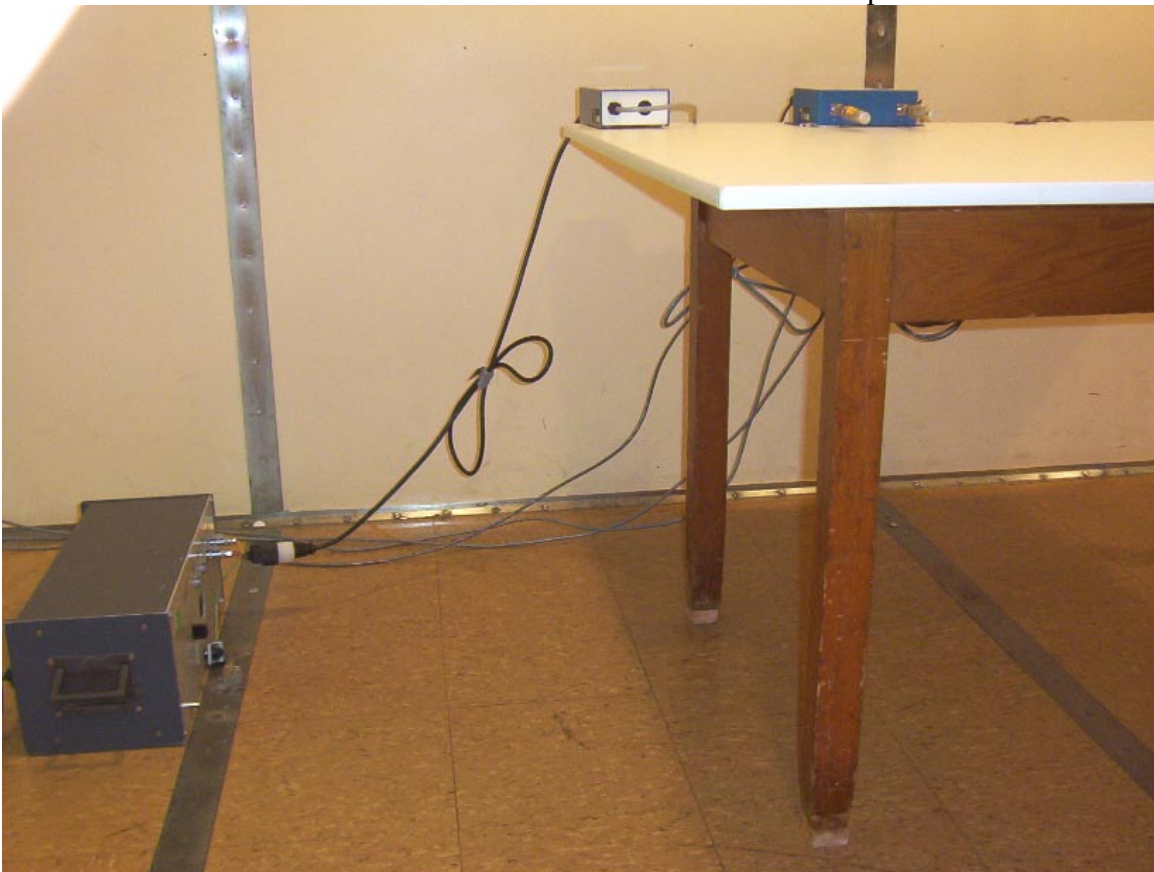
RFR-02/RFA-03 Radiated Emission Test Setup
