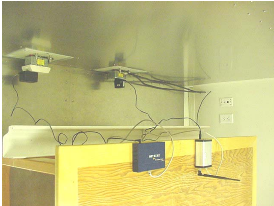
Photograph D.6-2 - AC Powerline Conducted Emissions Cable Placement
