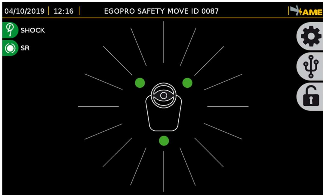
With this device, the system can acquire the three components of the acceleration vector ( $A_x$ ,  $A_y$ ,  $A_z$ ) that will be used to determine whether a shock was detected or not.
