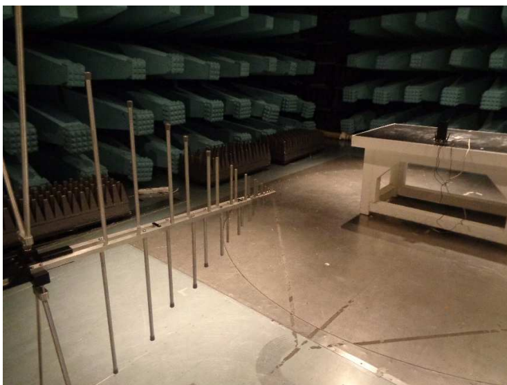
Radiated emission below 1 GHz – Antenna configuration 2
