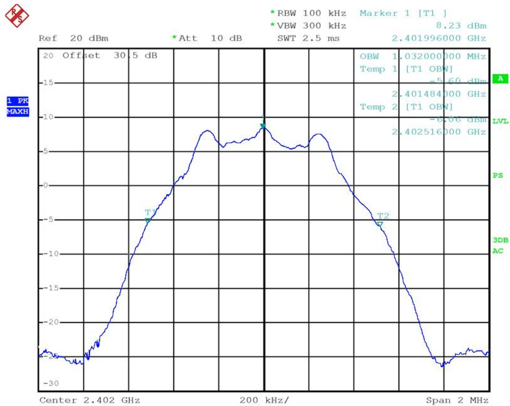
Figure 8.5-4: 99% occupied bandwidth on 802.11b, channel LOW
