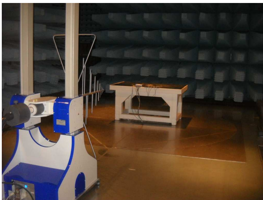
Radiated emission below 1 GHz with EUT in configuration 2
