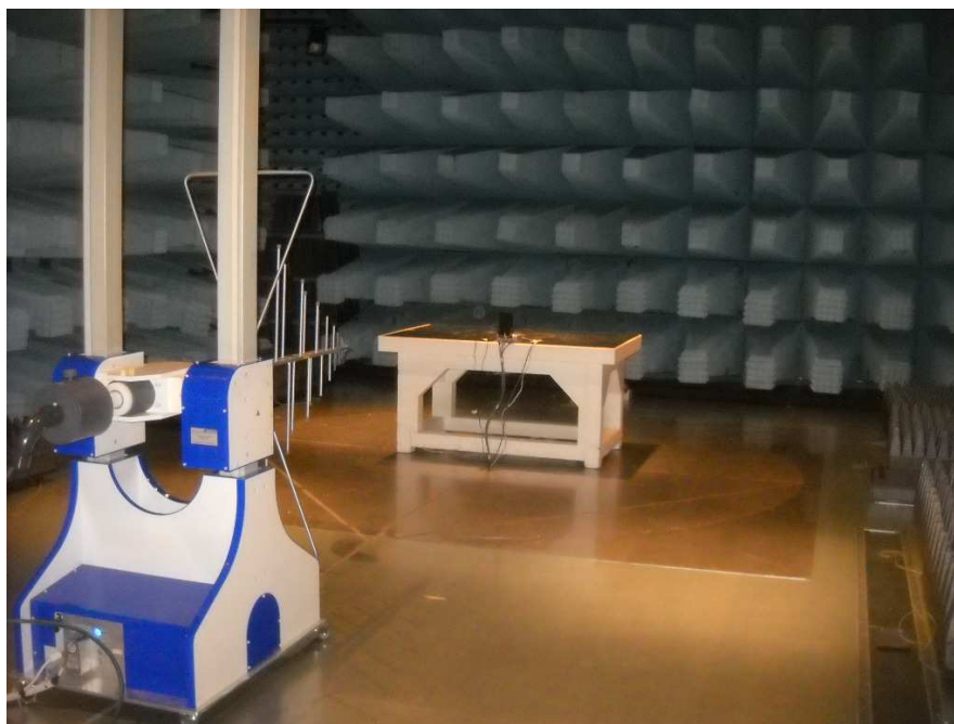
Radiated emission below 1 GHz with EUT in configuration 1
