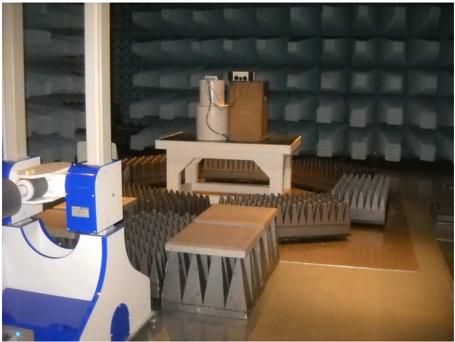
Radiated emission above 1 GHz with EUT in configuration 3
