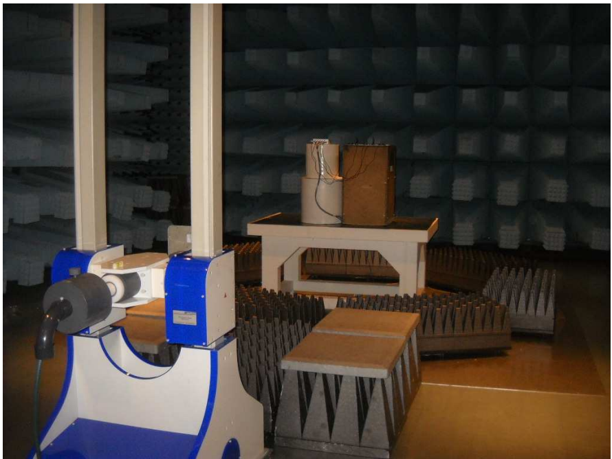
Radiated emission above 1 GHz with EUT in configuration 2
