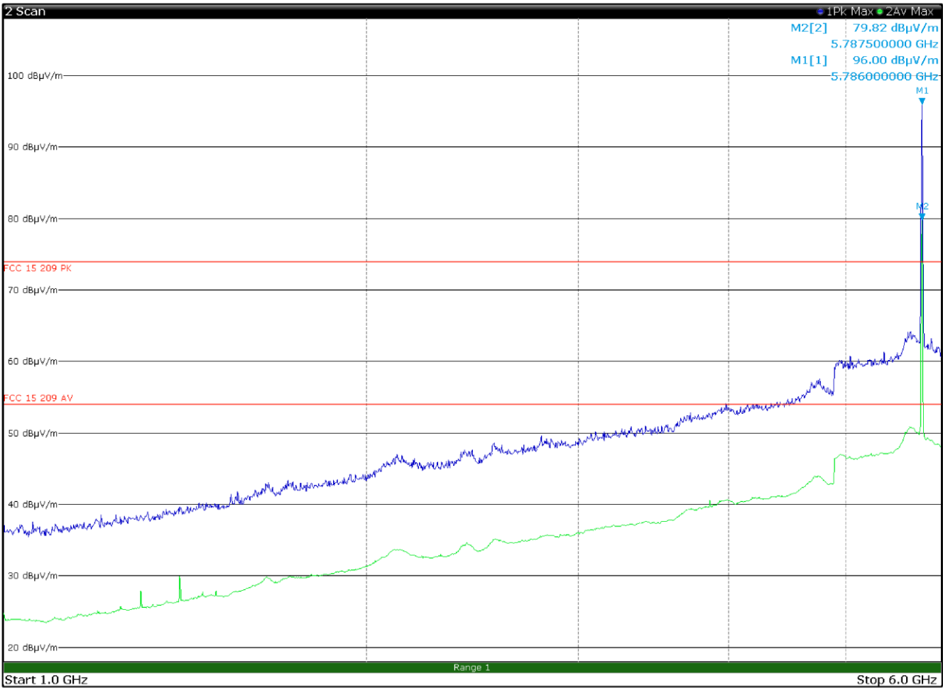
Figure 7.4-9: Radiated spurious emissions 1 to 6 GHz, 5785 MHz with antenna in horizontal polarization Limit exceeded by the carrier
