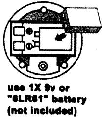
Insert one 9v or "SLR61" battery into the stadium-like controller. It requires total two batteries for two controllers. And then turn the switch to "On", where is located on the top of the batteries socket.
