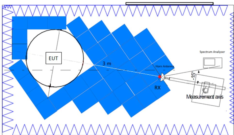
Radiated measurements setup  $f > 17$  GHz:
