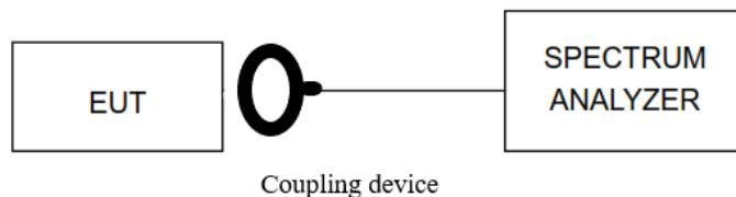
For frequency stability test the EUT was placed inside a climatic chamber and connected to a frequency meter using a low loss cable and a coupling device. An external DC power supply was connected to the EUT for voltage variation test.
