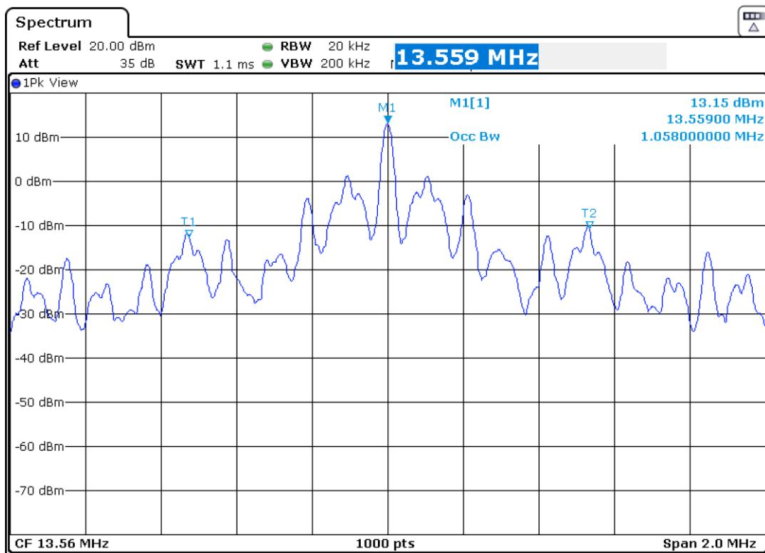
**Section 15.225 Subclause (a) / RSS-210 Clause B.6 (a). Field strength of emissions within the band 13.553 MHz -13.567 MHz**
