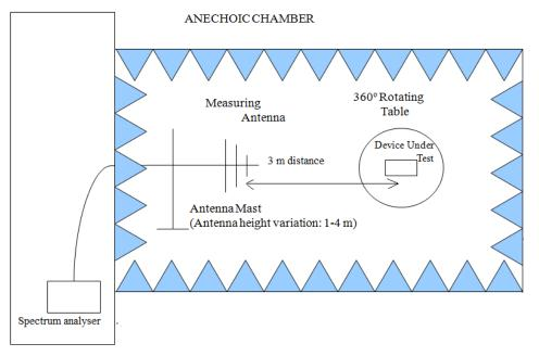
Shielded Control Room For Radiated Measurements
