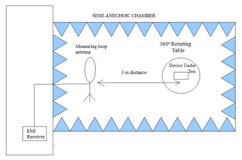
Shielded Control Room For Radiated Measurements
