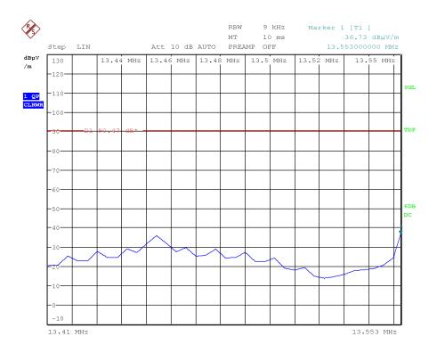
Note: The limit shown in the above plot is extrapolated to 3 meters
