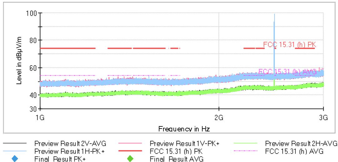
The peak above the limit is the Bluetooth LE carrier frequency.
