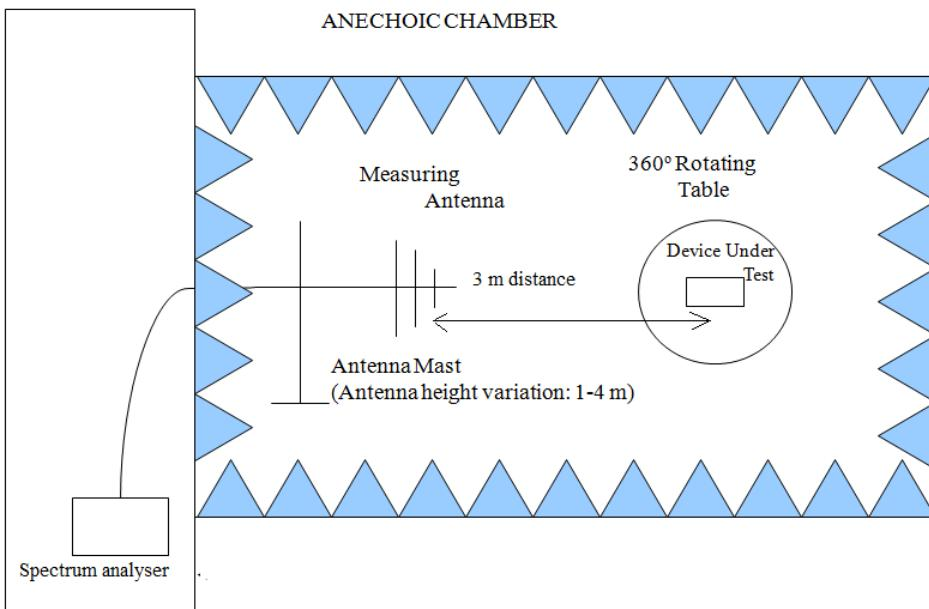
Radiated measurements setup  $f > 1$  GHz up to 17 GHz:
