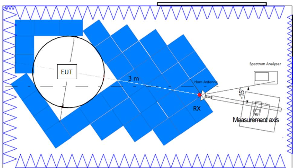
Radiated measurements setup  $f > 17$  GHz:
