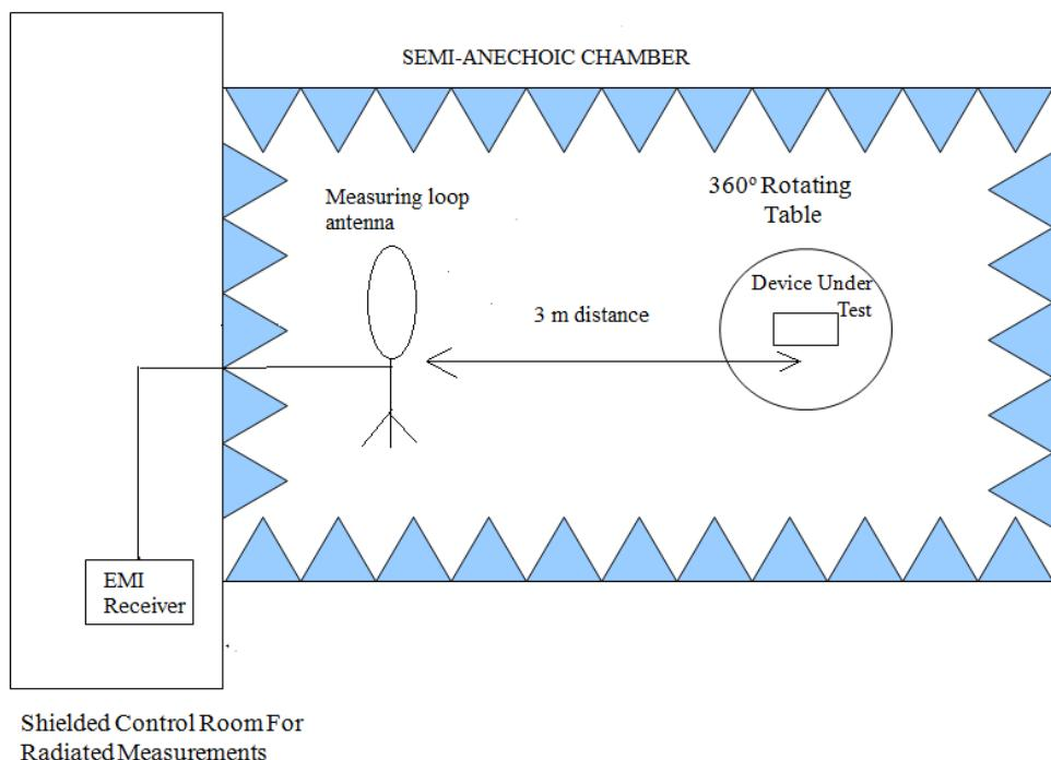
Radiated measurements setup 30 MHz to 200 MHz:
