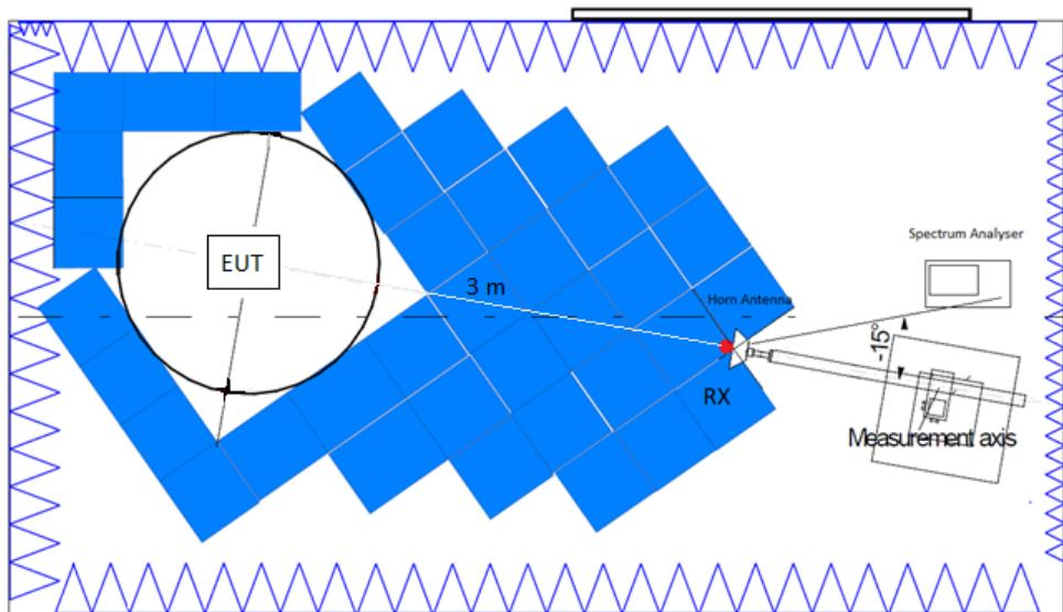
Radiated measurements setup  $f > 17$  GHz:
