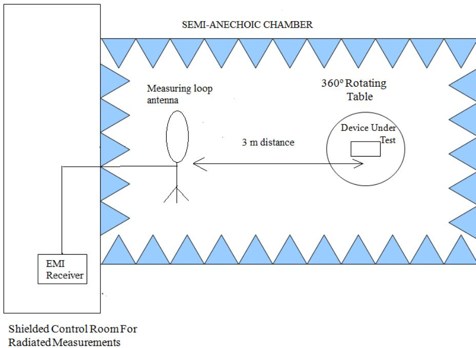
Radiated measurements setup  $30 \text{ MHz} < f < 1 \text{ GHz}$ :
