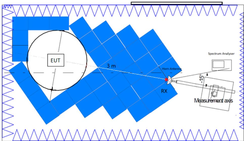
Radiated measurements setup  $f > 17$  GHz:
