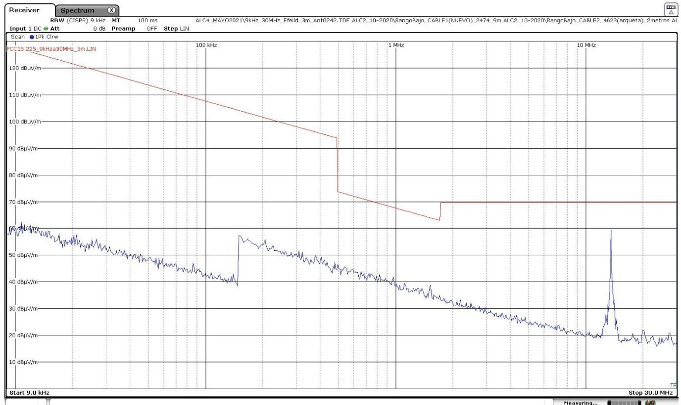
The highest peak is the NFC 13.56 MHz carrier frequency.
