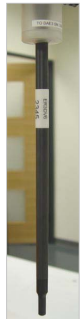
Figure 4 and 5: ER3DV6 E-Field Probe
