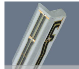
Figure 4 and 5: ER3DV6 E-Field Probe
