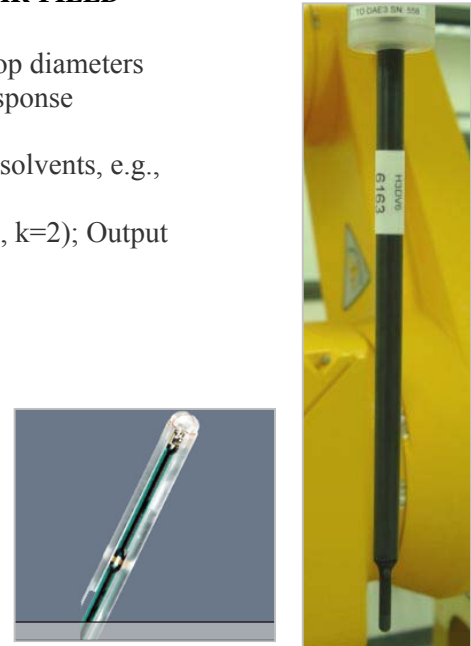
Figure 6 and 7: H3DV6 H-Field Probe
