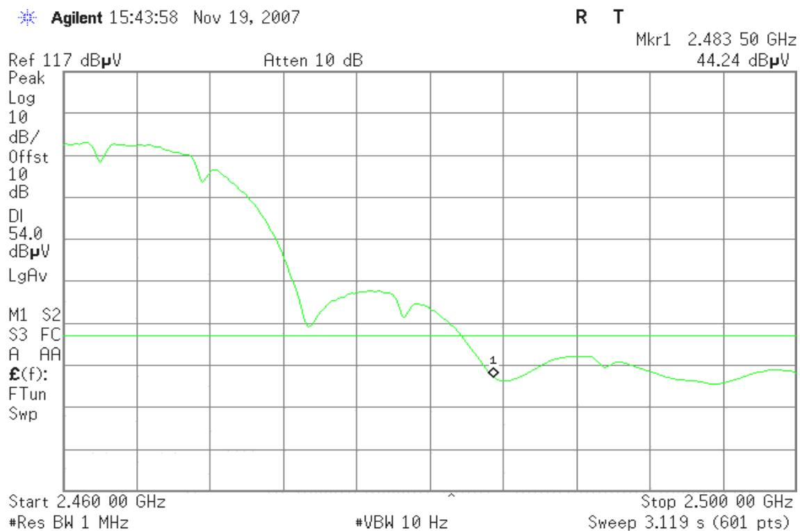
**Band Edges (IEEE 802.11g / CH Low)****Detector mode: Peak****Polarity: Vertical**
