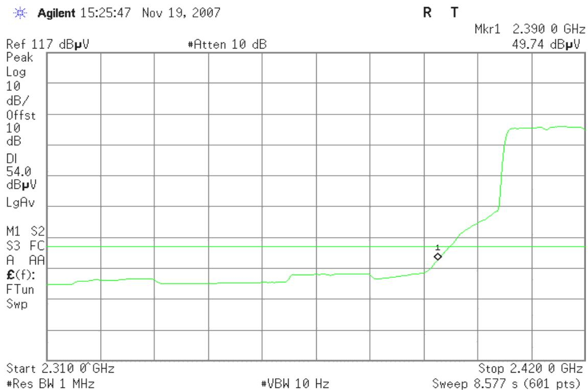
**Band Edges (IEEE 802.11g / CH High)****Detector mode: Peak****Polarity: Vertical**
