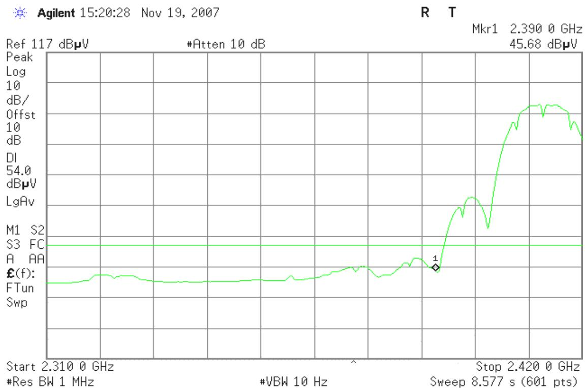
**Band Edges (IEEE 802.11b / CH High)****Detector mode: Peak****Polarity: Vertical**
