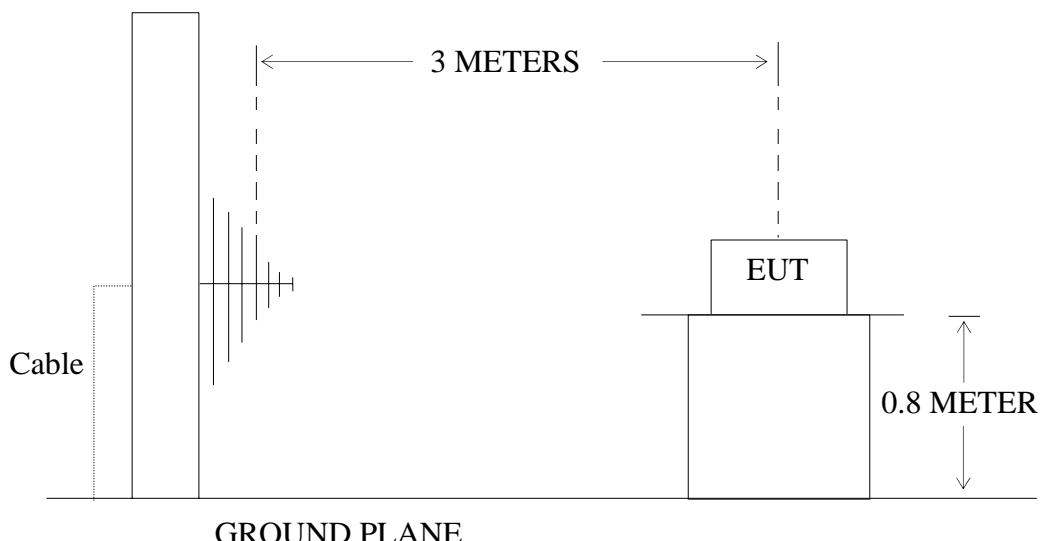
(EUT: Radio Frequency Presenter Laser Pointer)
