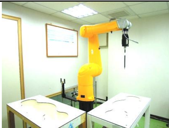
Fig-3.2 SPEAG DASY52 System
