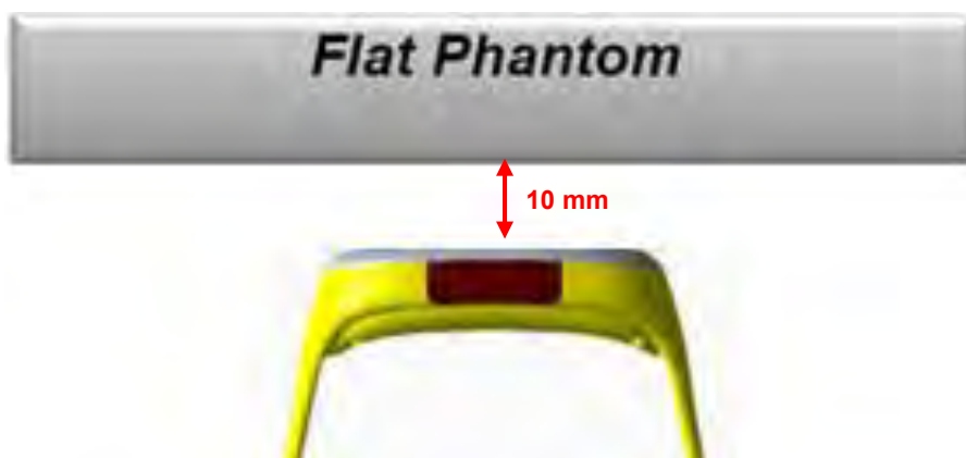
Fig-4.2 Illustration for Face Exposure Setup
