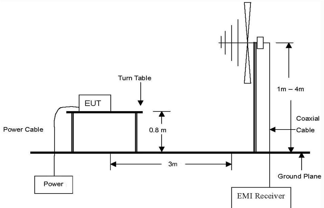
The diagram below shows the test setup that is utilized to make the measurements for emission .The spurious emissions were investigated form 1 GHz to the 10th harmonic of the highest fundamental frequency or 40 GHz, whichever is lower.
