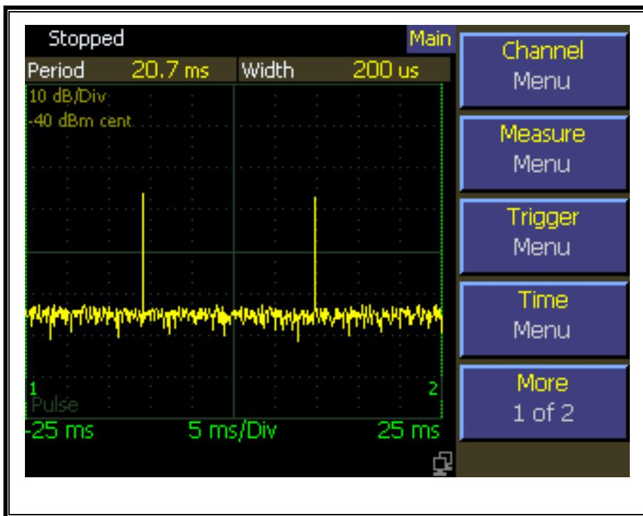
Note: Pulse width measurement has limited resolution in 5 ms/Div scan.
